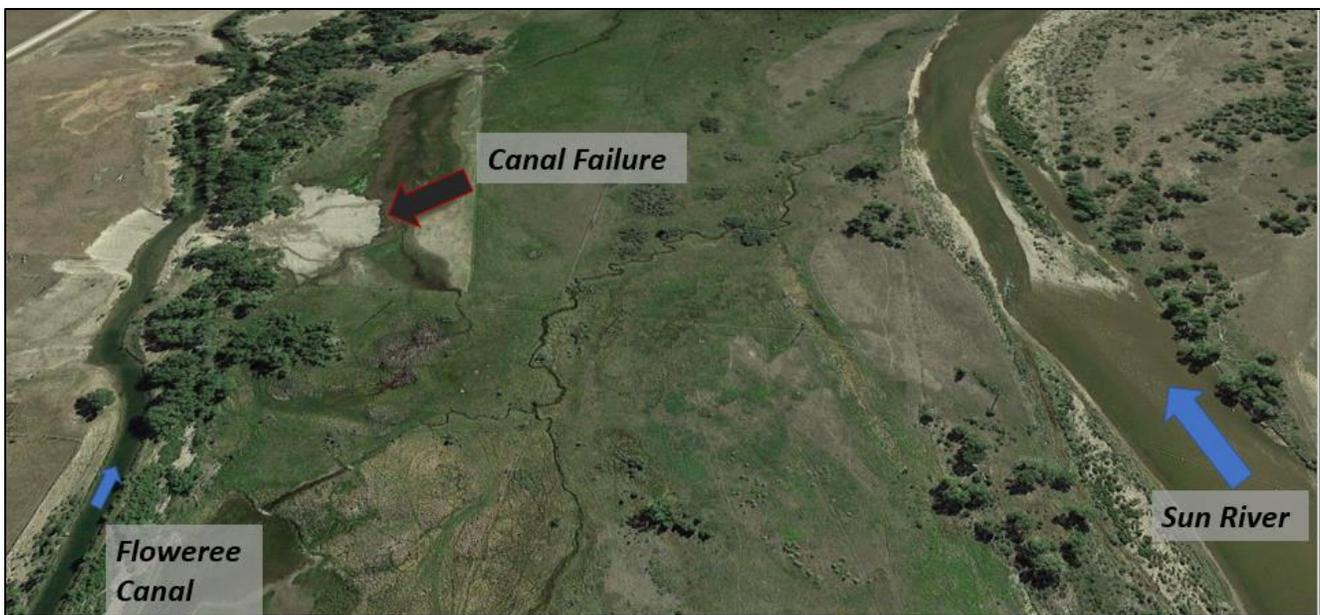
Figure 58. View downstream showing Floweree Canal breach forming alluvial fan on Sun River floodplain (Google Earth).
