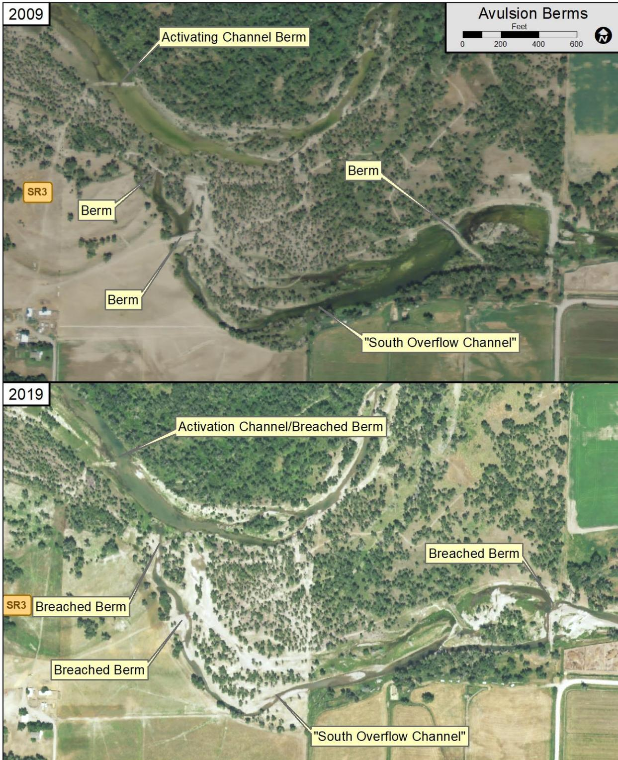
Figure 76. Activating channels on south floodplain about 1.5 miles upstream of Rocky Reef Diversion showing breaching of cross-channel berms between 2009 and 2019.
