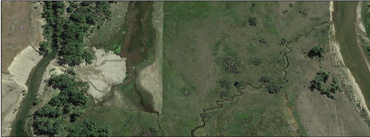
Figure 10. Google Earth photo showing Floweree Canal hillslope failure causing canal breach (left); Sun River is to right.
