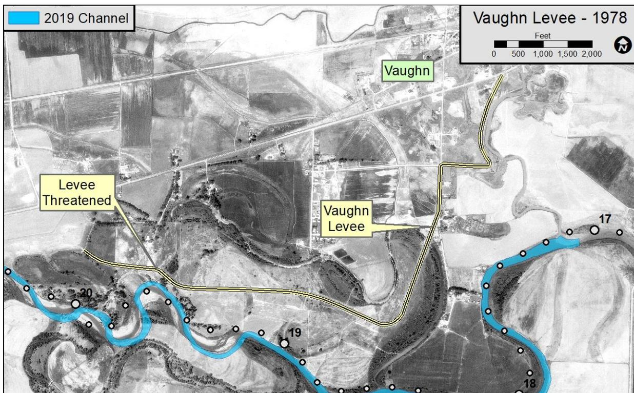
Figure 32. Vaughn Levee showing conditions a decade after it was built (1978 air photo); blue shows 2019 Sun River course and highlights large meander approaching and threatening levee.
