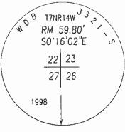
SET REBAR WITH ALUMINUM CAP AS SHOWN ABOVE.
