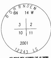
SET REBAR WITH ALUMINUM CAP AS SHOWN ABOVE.
