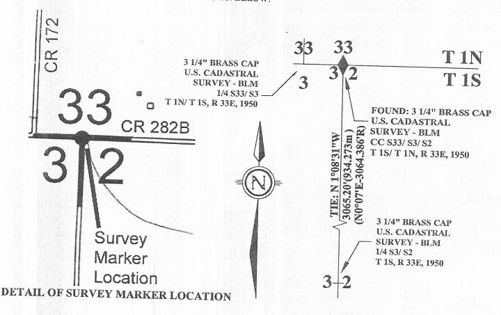
FND= 0.28' (0.085m) BLM BC /0.89' (0.27m) BELOW ASP RD CTY RD 282B @ "T" INTER /RM SW FND S. D. Signature Photonia Part Chief y represents with performed by e with the the Corner TAND Date: 11-18-01 Reg. No. 145/645 SKETCH OF CORNER
