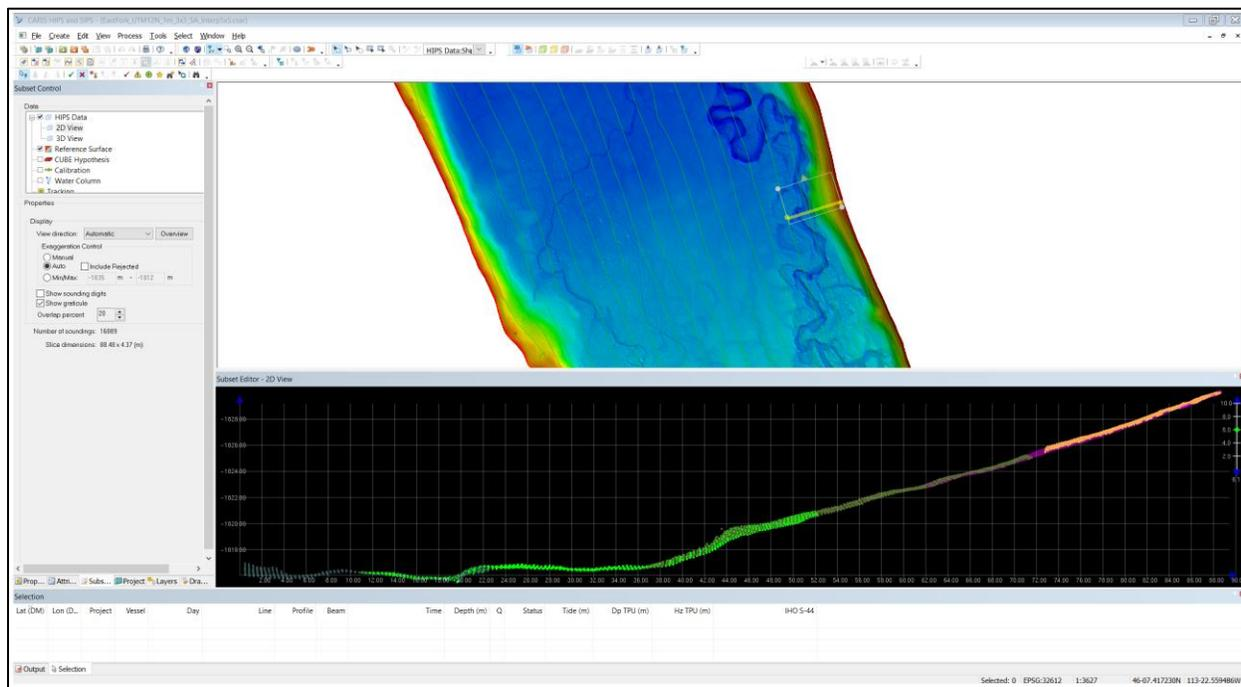
Figure 10: Multibeam Editing in Subset Mode for East Fork
