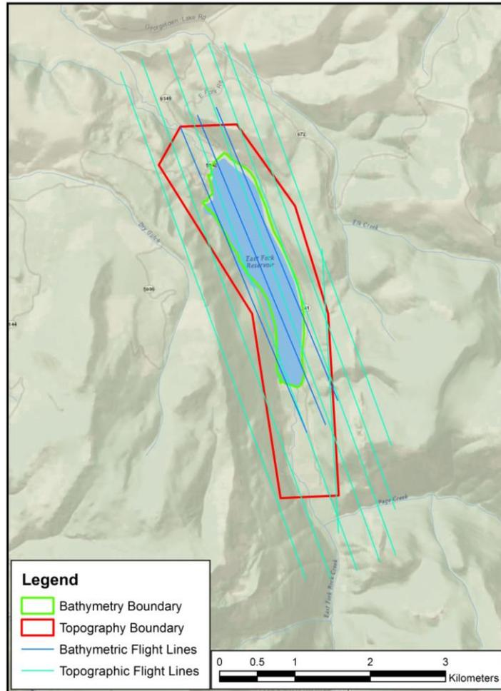
Figure 4: East Fork Planned Flight Lines
