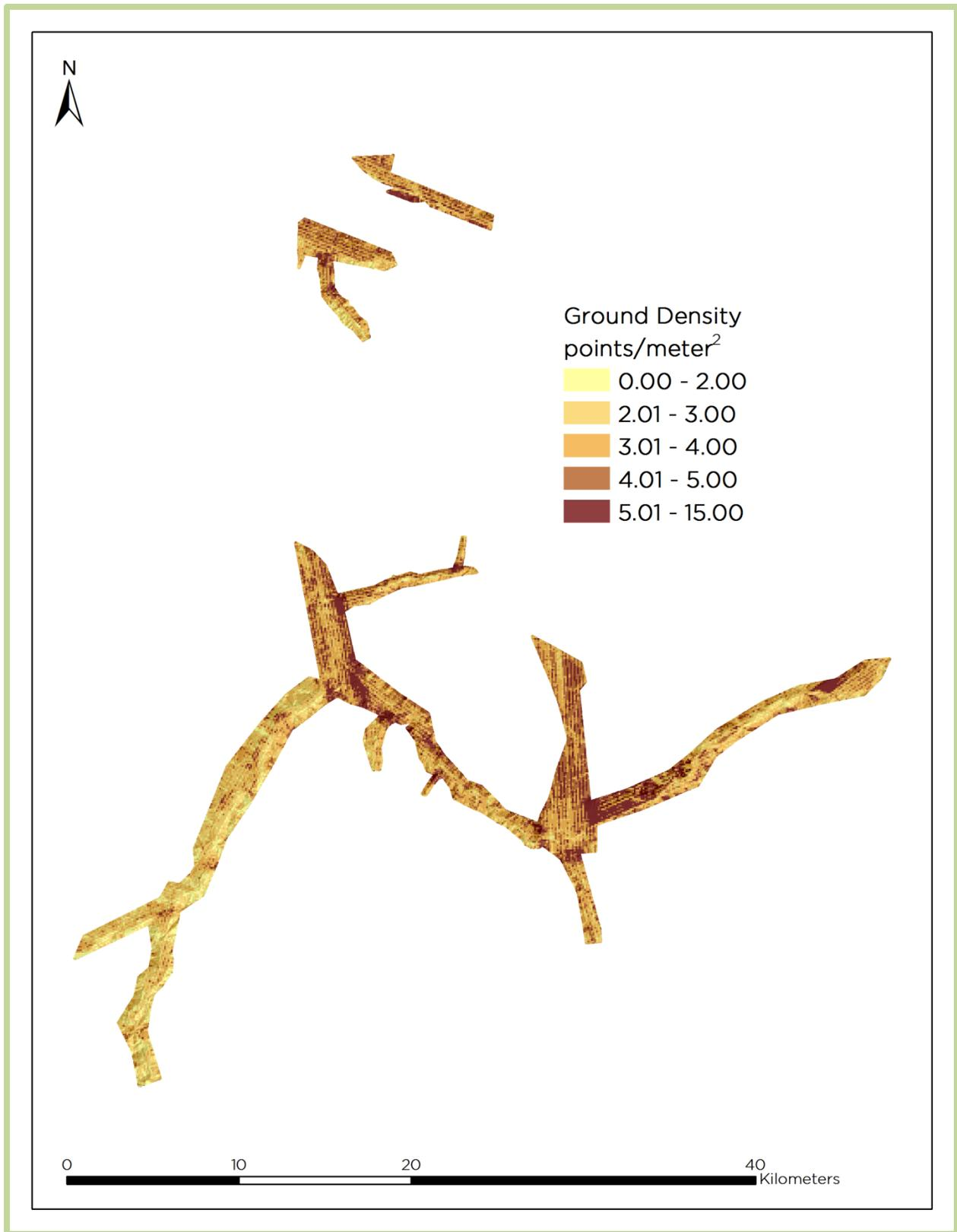
**Figure 7: Ground density map for the Ravalli County LiDAR - Phase III site**
