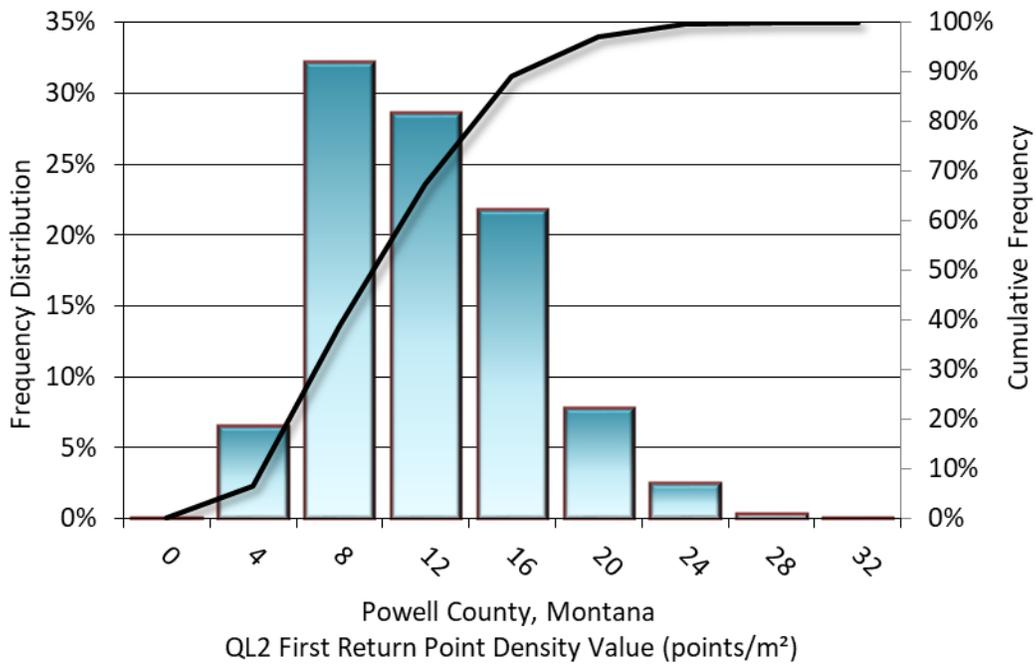
**Figure 8: Frequency distribution of first return point density values in the QL2 dataset per 100 x 100 cells**
