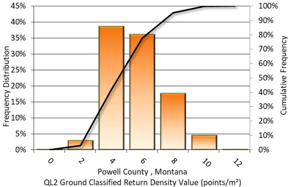
**Figure 9: Frequency distribution of ground classified return density values in the QL2 dataset per 100 x 100 m cells**
