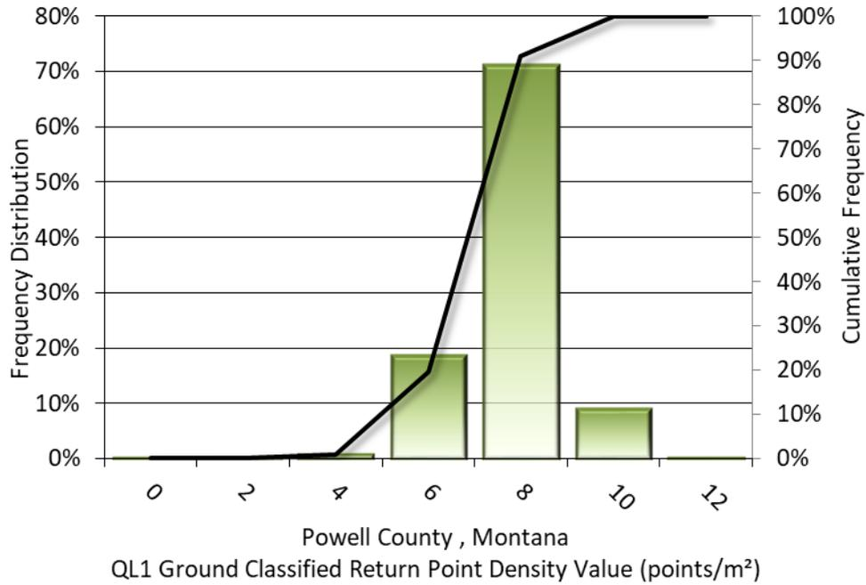
**Figure 7: Frequency distribution of ground classified return density values in the QL1 dataset per 100 x 100 m cells**
