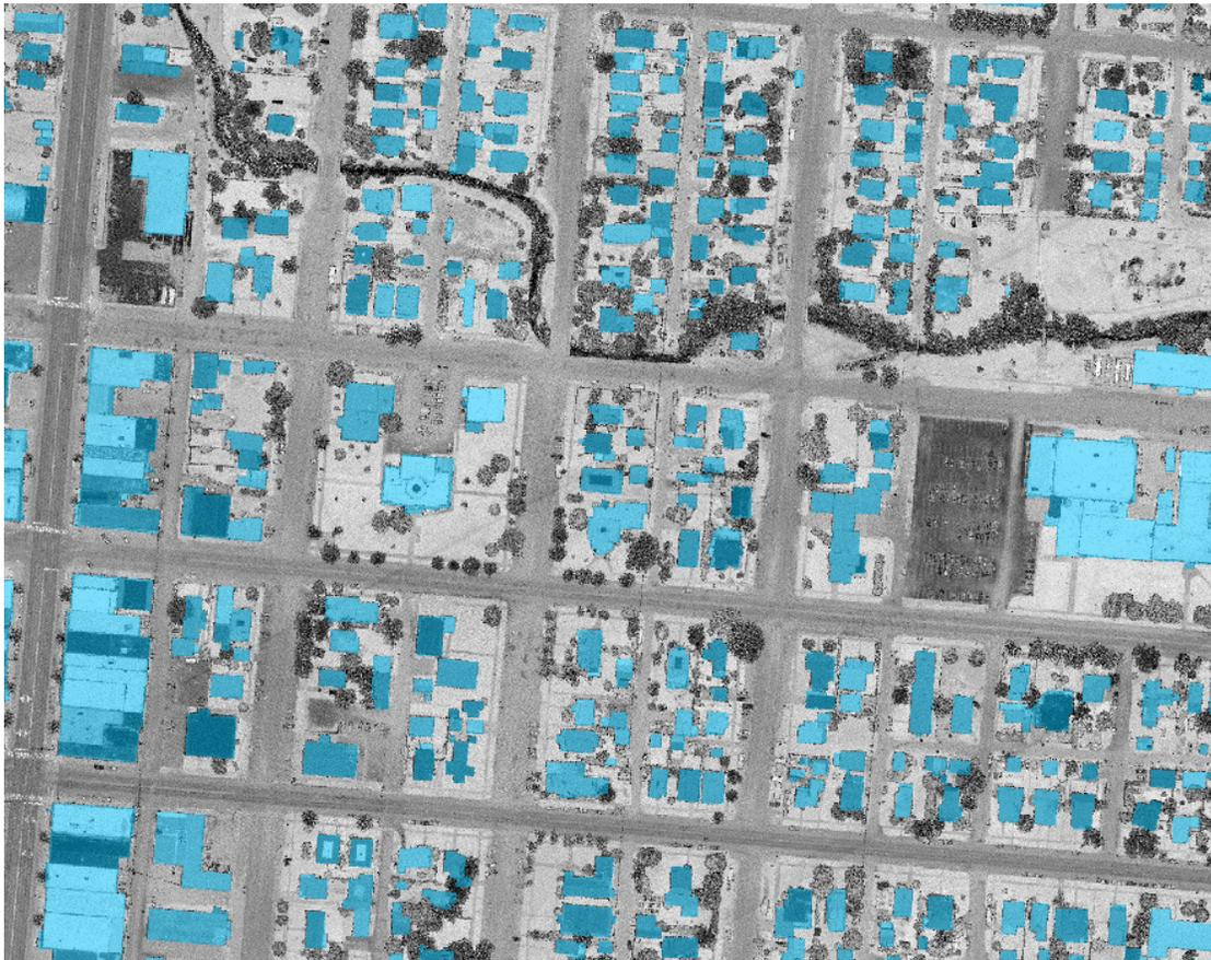
**Figure 5: This aerial view of the lidar point cloud is colored by intensity and is overlaid with the 3D building footprint in the Powell County dataset**
