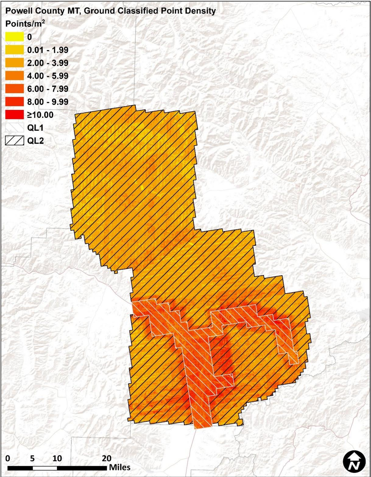
Figure 11: Ground-classified point density map for the Powell County site (100 m x 100 m cells)
