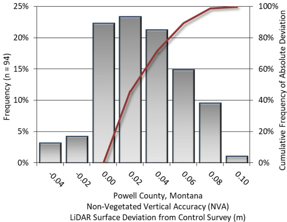
**Figure 12: Frequency histogram for the Lidar unclassified LAS deviation from ground check point values (NVA)**
