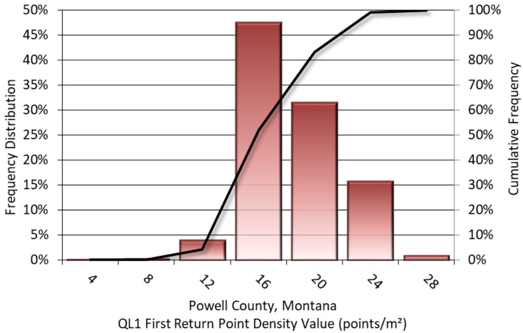
**Figure 6: Frequency distribution of first return point density values in the QL1 dataset per 100 x 100 m cells**
