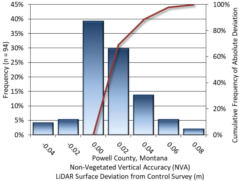
**Figure 13: Frequency histogram for Lidar bare earth DEM surface deviation from ground check point values (NVA)**
