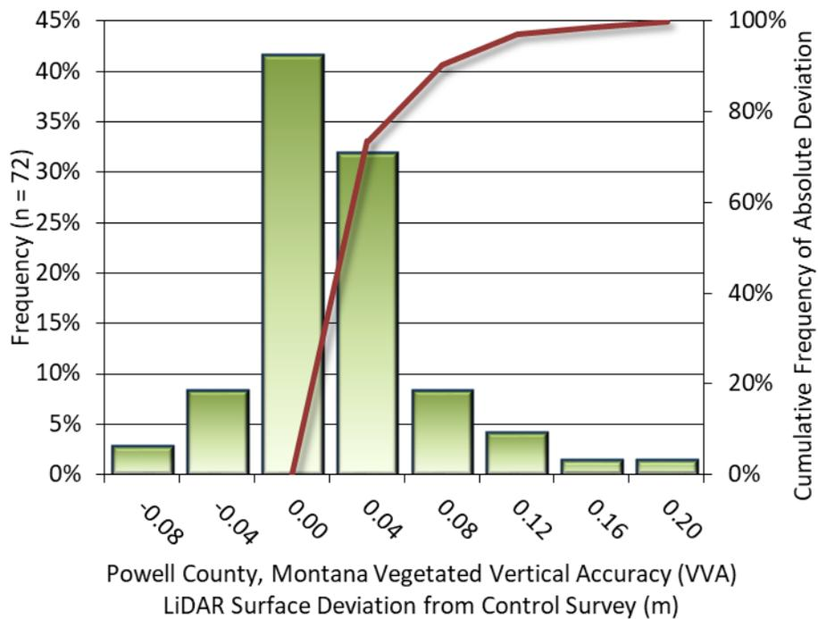
**Figure 15: Frequency histogram for Lidar surface deviation from vegetated check point values (VVA)**
