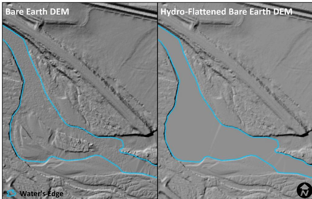
**Figure 3: Example of hydroflattening in the Powell County Lidar dataset**
