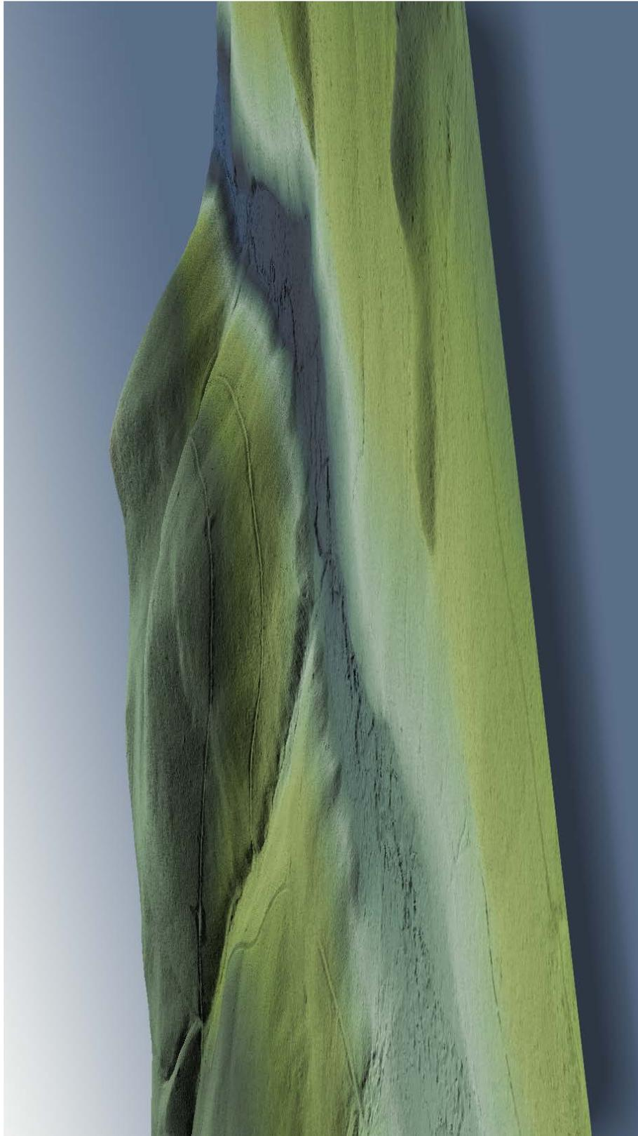
**Figure 15: View looking East down Hope Creek. The image was created from the gridded LiDAR surface colored by elevation.**
