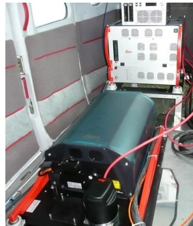
**Leica ALS70 LiDAR sensor**
