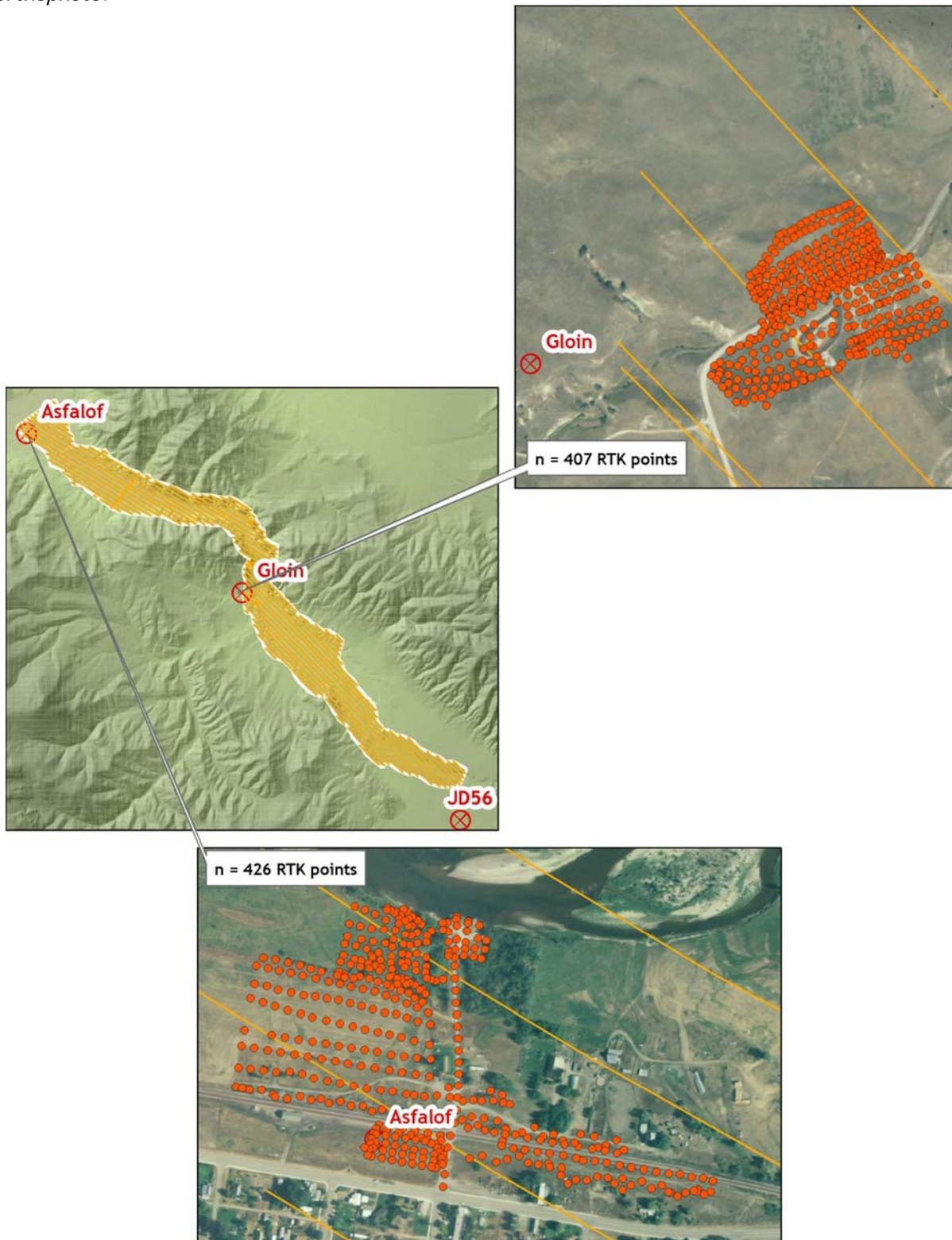
Figure 2.11. Selected RTK point locations from Maddy River study area displayed on a NAIP orthophoto.
