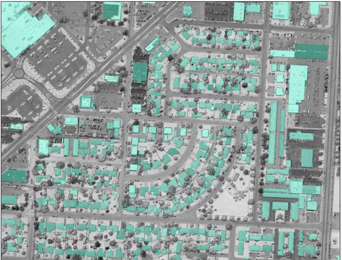
**Figure 3: Example of building footprint feature extraction, created from the Clark Fork Bitterroot above-ground LiDAR point cloud colored by intensity, overlaid with the 3D building polygon**
