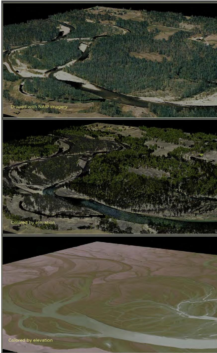
**Figure 10: View looking east at the Bitterroot River. The top image is the 3D LiDAR point cloud draped with NAIP imagery, the center image is the LiDAR point cloud colored by elevation, the bottom image is the gridded bare earth model colored by elevation.**
