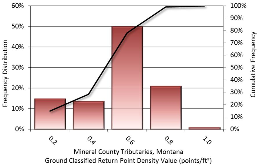
**Figure 8: Frequency distribution of ground-classified return point density values of 2016-2017 acquisitions per 100 x 100 m cell**
