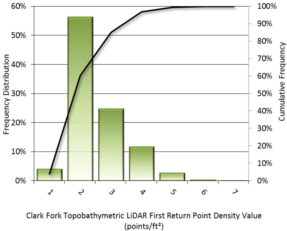
Figure 6: Frequency distribution of Clark Fork, Montana first return densities per 100 x 100 m cell
