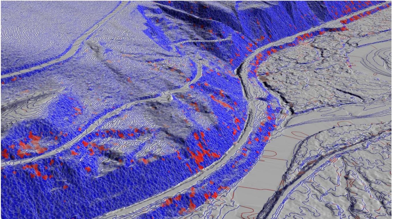
**Figure 3: 1-foot contours draped over the St. Regis River bare earth elevation model. Blue contours represent high confidence while the red contours represent low confidence.**
