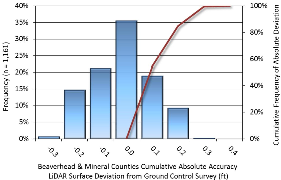
Figure 12: Frequency histogram for LiDAR surface deviation from QSI's ground control point values
