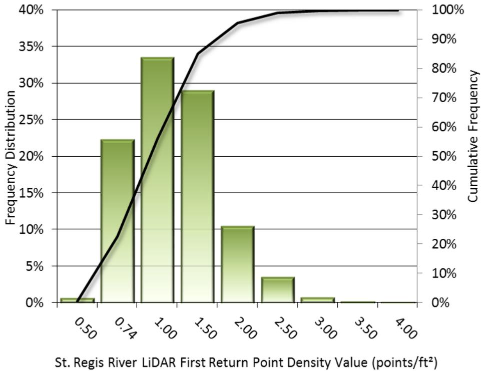
Figure 5: Frequency distribution of St. Regis River, Montana first return densities per 100 x 100 m cell
