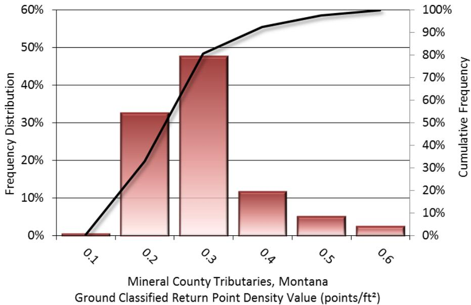
**Figure 6: Frequency distribution of ground-classified return point density values of 2019 acquisition per 100 x 100 m cell**
