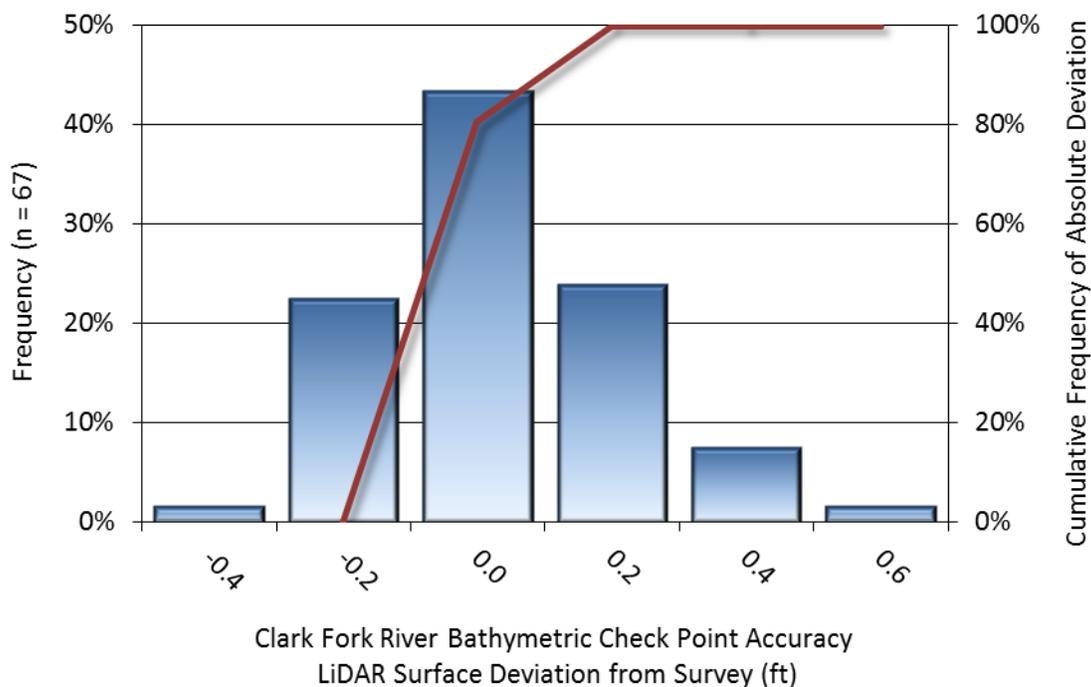
**Figure 14: Clark Fork River Frequency histogram for LiDAR surface deviation from bathymetric check point values**
