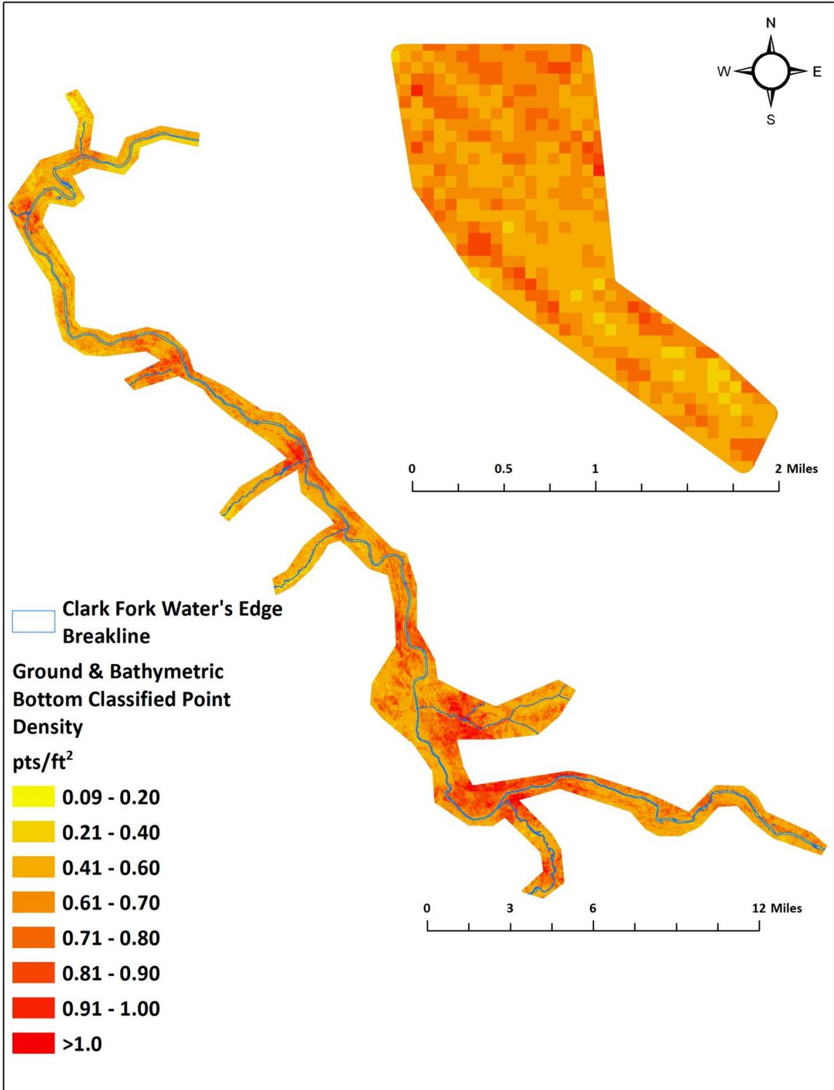
Figure 10: Ground & bathymetric bottom classified point density map for the Clark Fork & Lima sites (300 ft x 300 ft cells). Bathymetric bottom corresponds to areas inside Clark Fork water breaklines.
