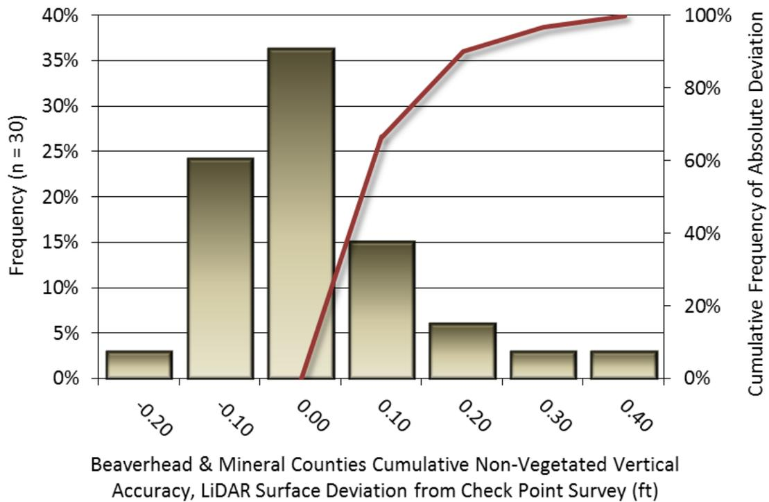
Figure 11: Frequency histogram for LiDAR surface deviation from non-vegetated check point values
