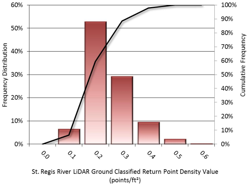
Figure 6: Frequency distribution of St. Regis River, Montana ground classified densities per 100 x 100 m cell
