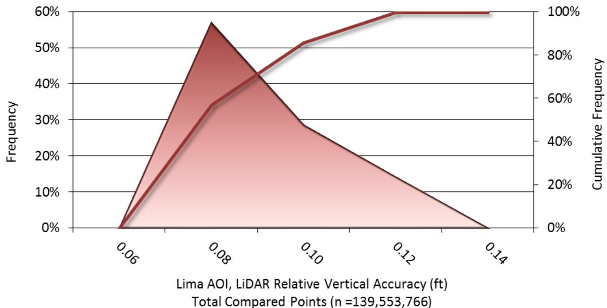
**Figure 15: Frequency plot for relative vertical accuracy between flight lines for the Lima AOI**
