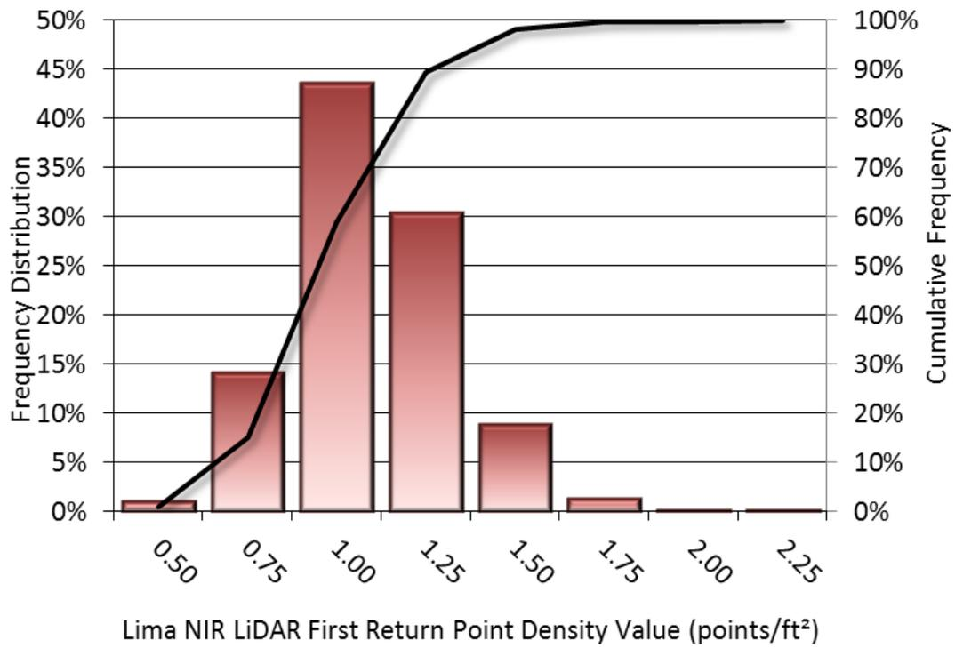
Figure 5: Frequency distribution of Lima, Montana first return densities per 100 x 100 m cell
