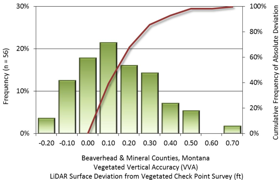
**Figure 10: Frequency histogram for LiDAR surface deviation from land cover class point values (VVA)**
