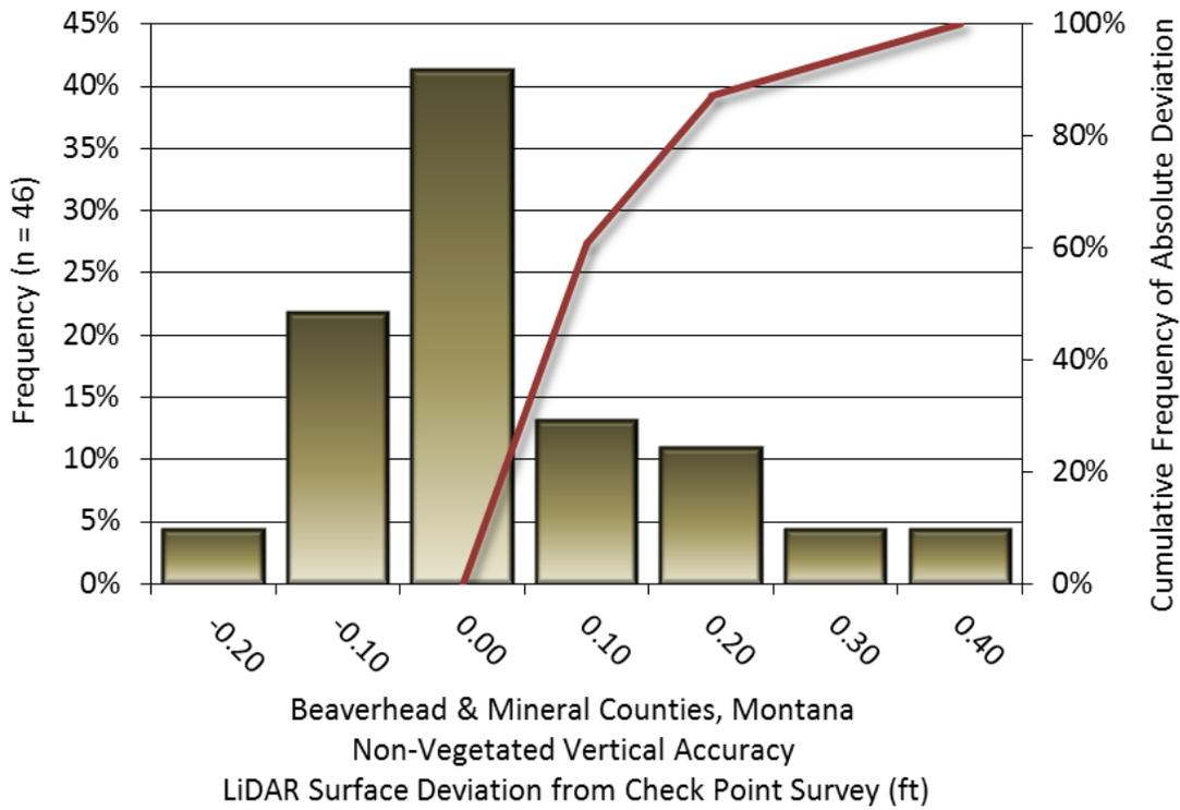
Figure 8: Frequency histogram for LiDAR surface deviation from non-vegetated check point values
