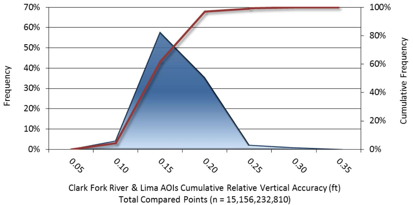
Figure 17: Cumulative frequency plot for relative vertical accuracy between flight lines
