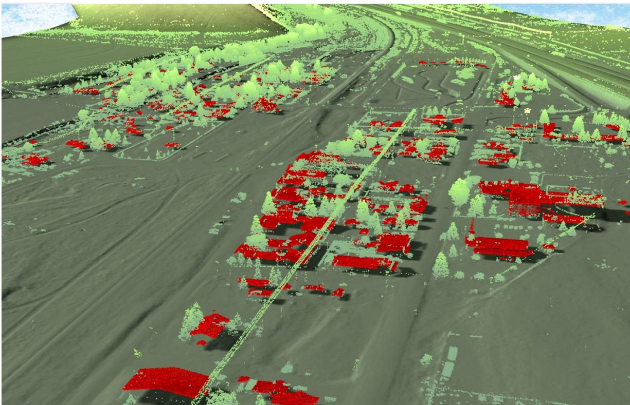
**Figure 4: This image shows a view of the building classification in the previously delivered Lima AOI, created from the bare earth model colored by elevation, and overlaid with the above-ground point cloud colored by point classification.**
