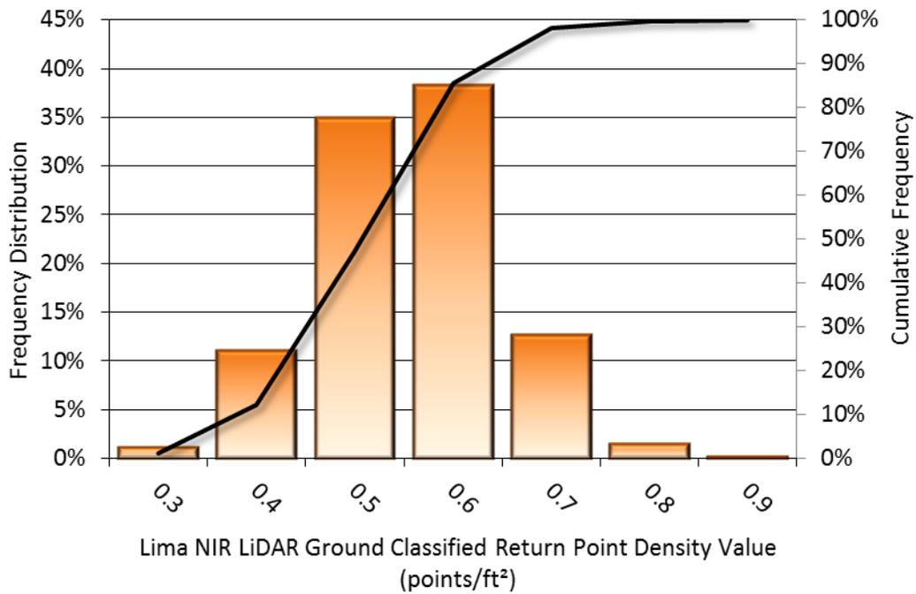
**Figure 8: Frequency distribution of Lima, Montana ground classified densities per 300 x 300 ft cell**
