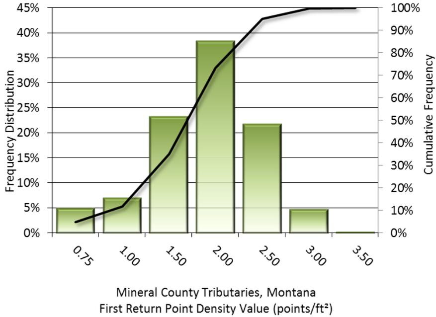
**Figure 7: Frequency distribution of first return point density values of 2016-2017 acquisitions per 100 x 100 m cell**
