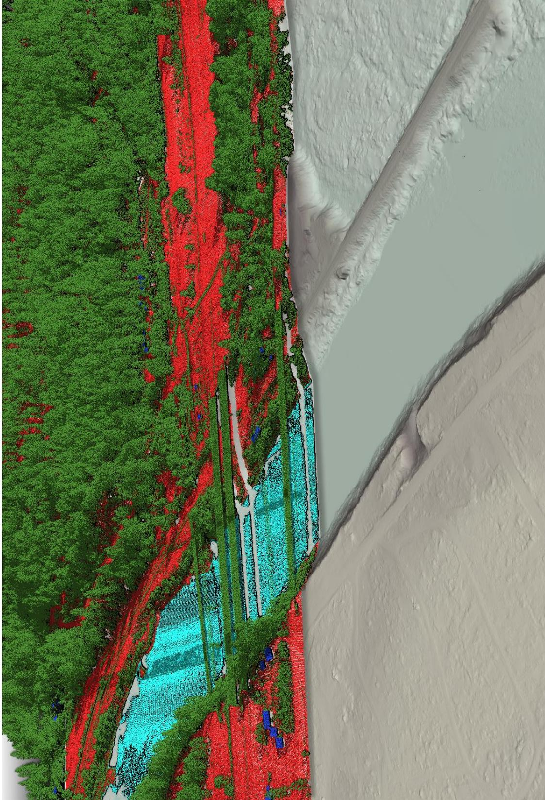
**Figure 13: This image shows another view of the St. Regis River bare earth DEM, overlaid with above ground returns colored by point classification in half of the image.**
