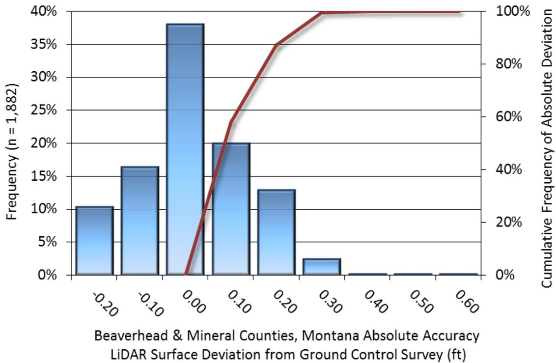
Figure 9: Frequency histogram for LiDAR surface deviation from QSI's ground control point values
