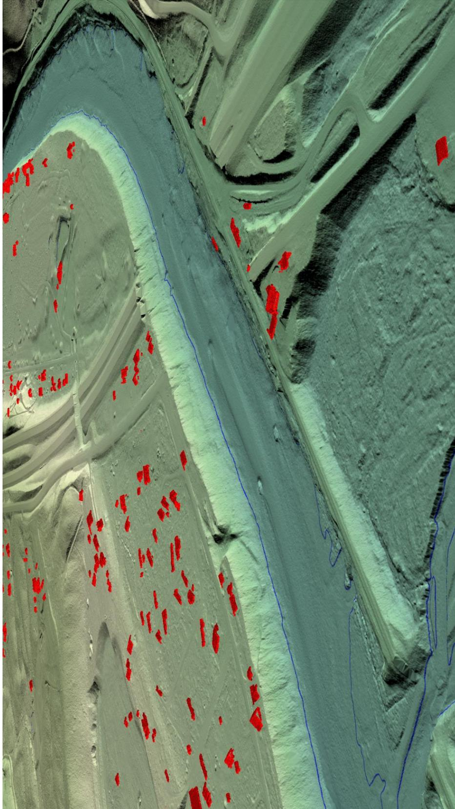
Figure 19: This image shows another view of the Clark Fork River topobathymetric bare earth DEM, with water's edge breaklines and building-classified LIDAR returns overlaid.
