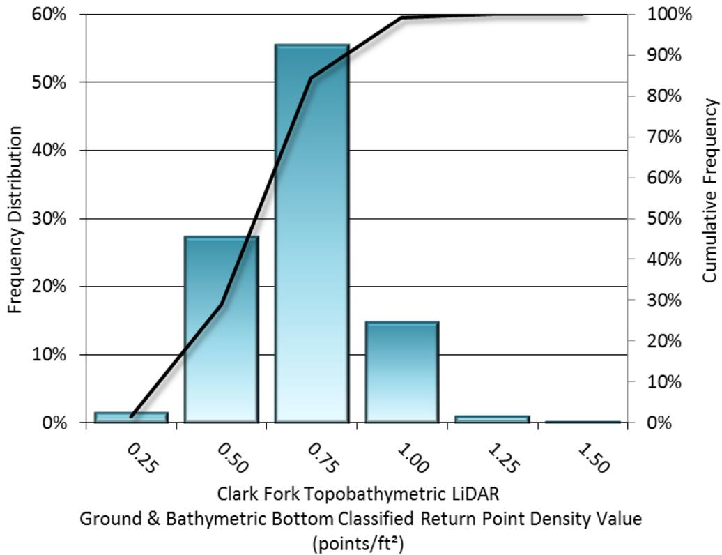
**Figure 9: Frequency distribution of Clark Fork, Montana ground and bathymetric bottom classified densities per 300 x 300 ft cell**
