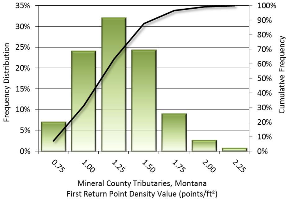
**Figure 5: Frequency distribution of first return point density values of 2019 acquisition per 100 x 100 m cell**
