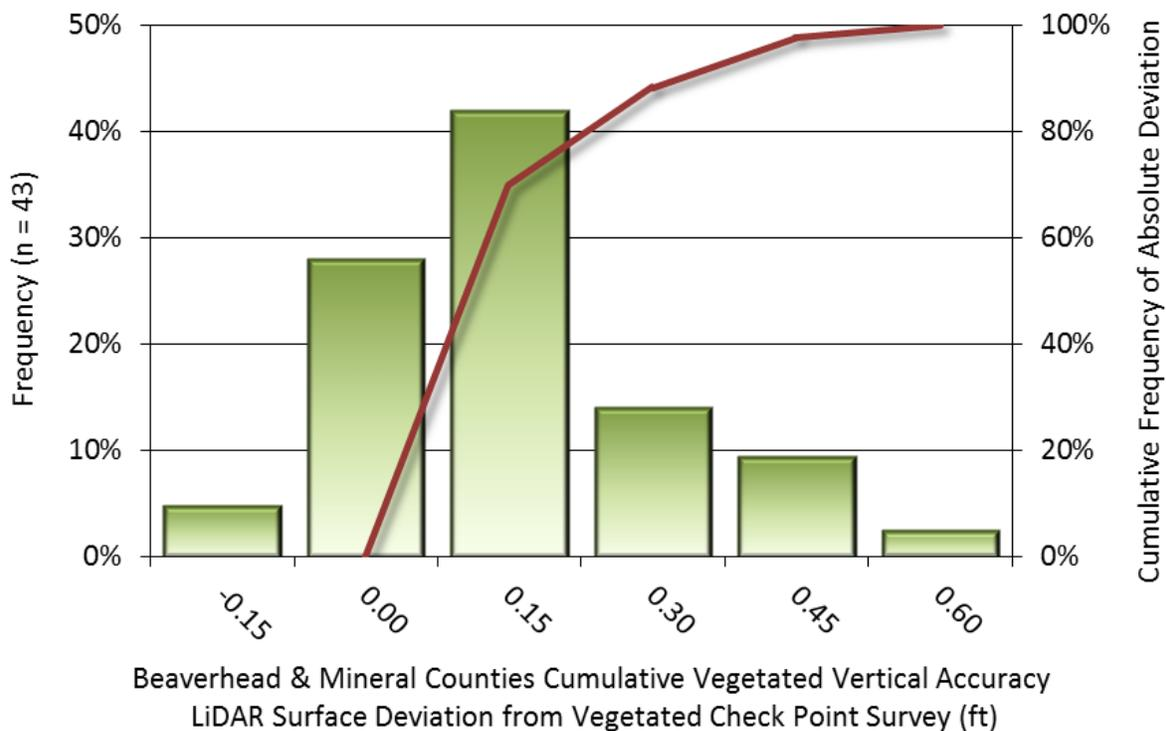
**Figure 13: Frequency histogram for LiDAR surface deviation from land cover class point values (VVA)**
