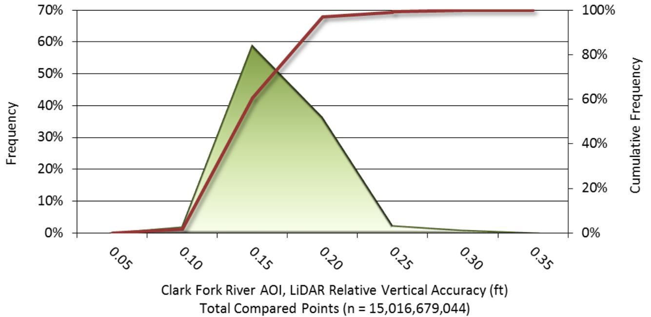
Figure 16: Frequency plot for relative vertical accuracy between flight lines for the Clark Fork AOI
