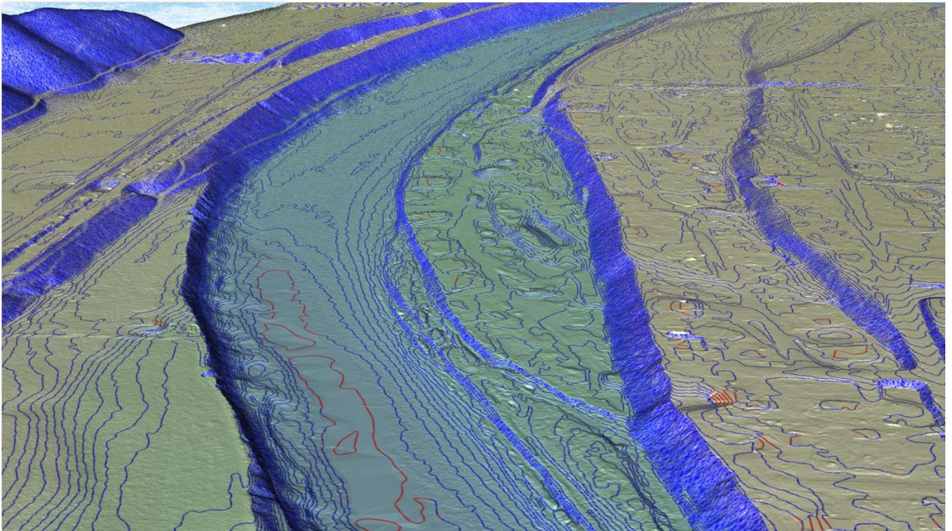
**Figure 3: 1-foot contours draped over the Clark Fork bare earth elevation model. Blue contours represent high confidence while the red contours represent low confidence.**
