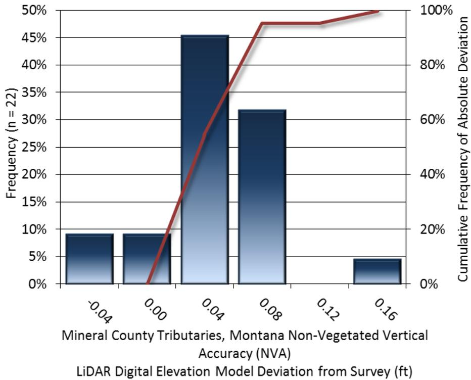
**Figure 13: Frequency histogram for LiDAR bare earth DEM surface deviation from ground check point values (NVA)**
