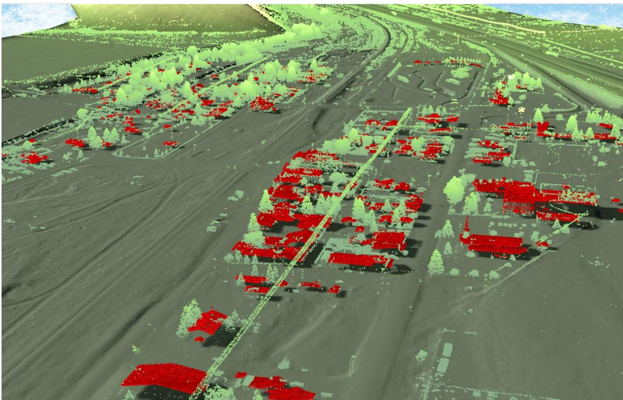
**Figure 4: This image shows a view of the building classification in the Lima AOI, created from the bare earth model colored by elevation, and overlaid with the above-ground point cloud colored by point classification.**
