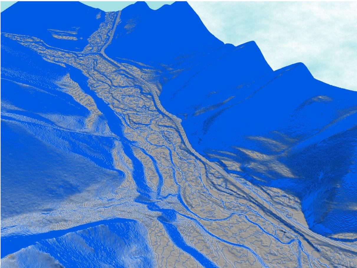
**Figure 4: Contours draped over the Mineral County Tributaries bare earth elevation model**
