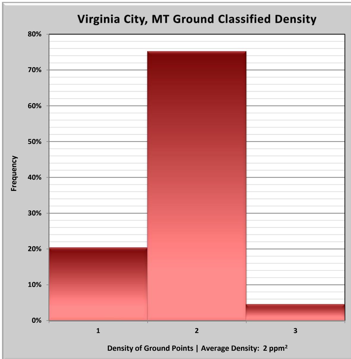
**Exhibit 12:** Ground Classified Laser Point Density by Tile, points/m<sup>2</sup>
