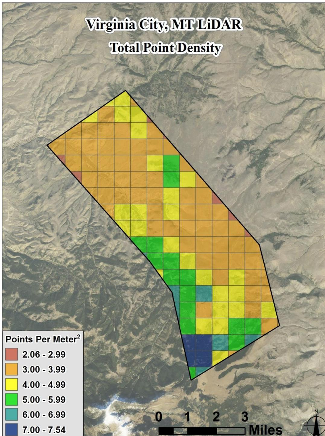
The following two exhibits show the density of **ground classified points**. Factors such as vegetation, water, and buildings will reduce the density of points classified to the ground. For the Virginia City, MT project, an average of **2** ground classified points per square meter was achieved.
