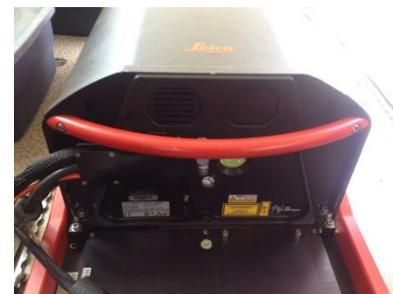
**Leica ALS80 LiDAR sensor**
