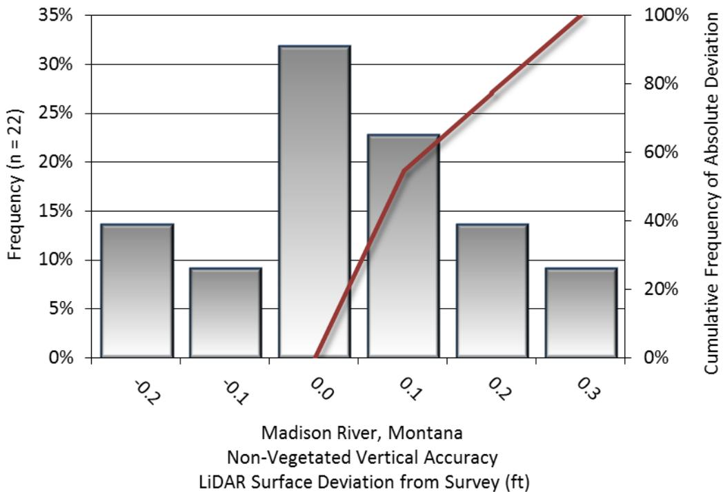
**Figure 9: Frequency histogram for LiDAR surface deviation from ground check point values (NVA)**
