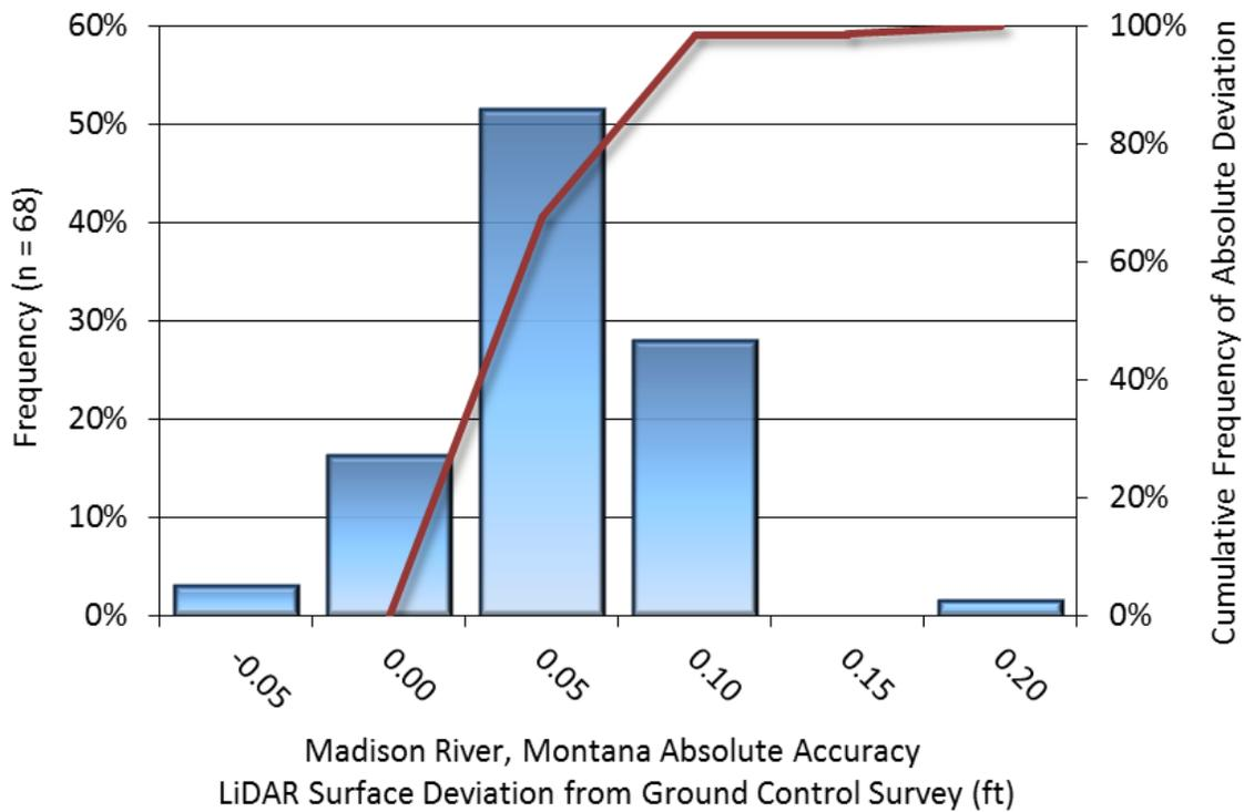
**Figure 11: Frequency histogram for LiDAR surface deviation from ground control point values**
