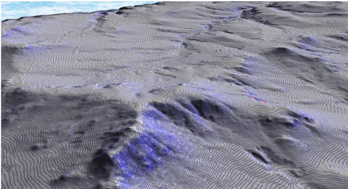
**Figure 4: Contours draped over the bare earth elevation model in one of the MTDNRC project sites. Blue contours represent high confidence while the red contour segments represent low confidence.**
