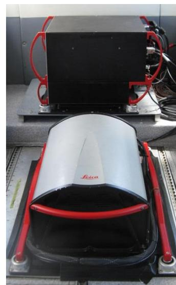
To reduce laser shadowing and increase surface laser painting, all areas were surveyed with an opposing flight line side-lap of  $\geq 50\%$  ( $\geq 100\%$  overlap). The Leica laser systems record up to four range measurements (returns) per pulse. All discernible laser returns were processed for the output dataset.
