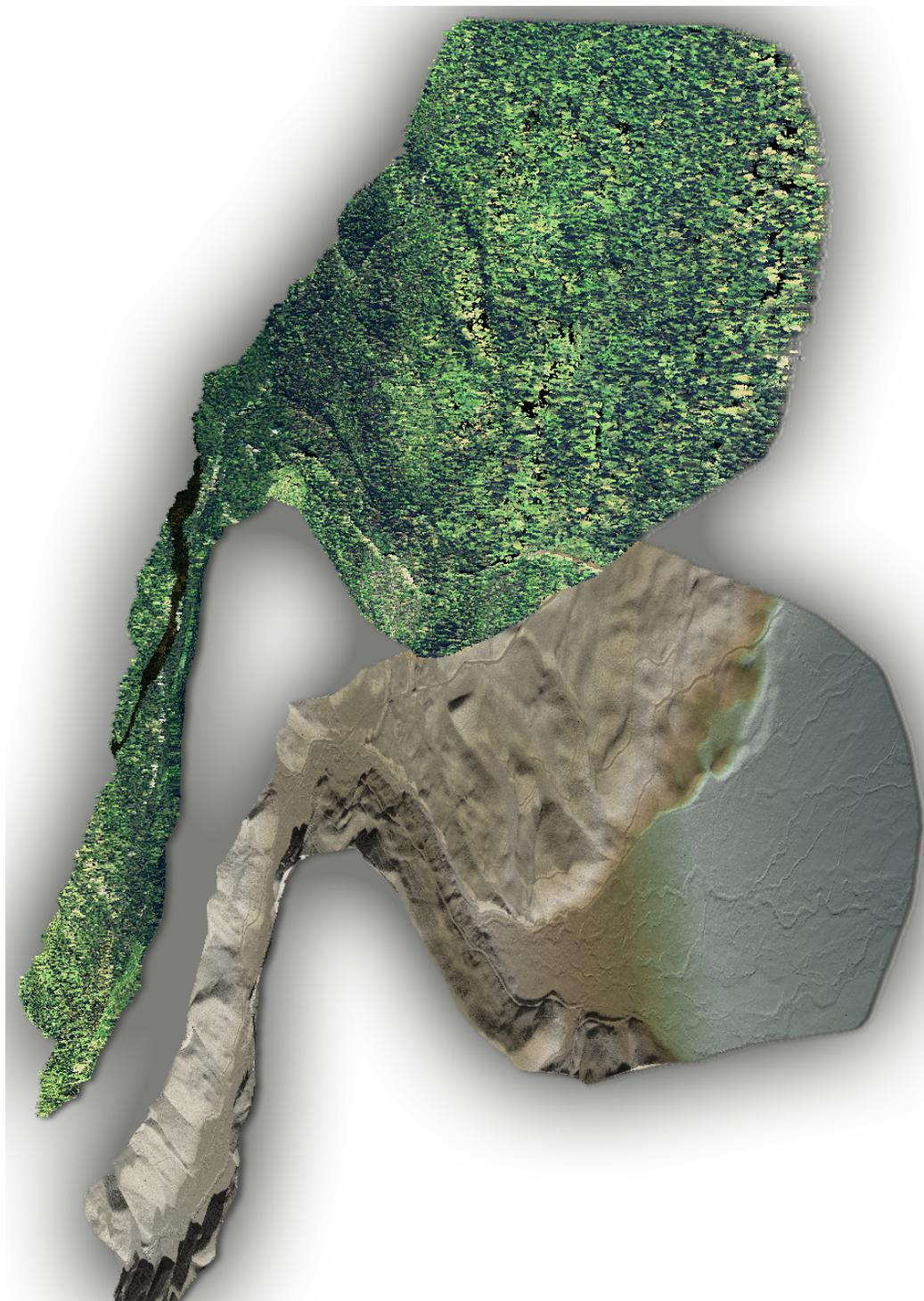
**Figure 10:** A Stacked view of the Cottonwood Creek AOI. The left image is the bare-earth model colored by elevation, the right image is the 3D LiDAR point cloud draped with NAIP imagery.
