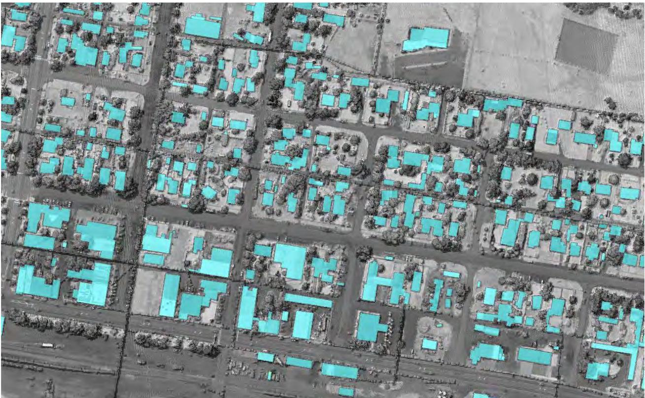
**Figure 3: This aerial view of the lidar point cloud is colored by intensity, and is overlaid with the 3D building footprint in the Jefferson County project area.**
