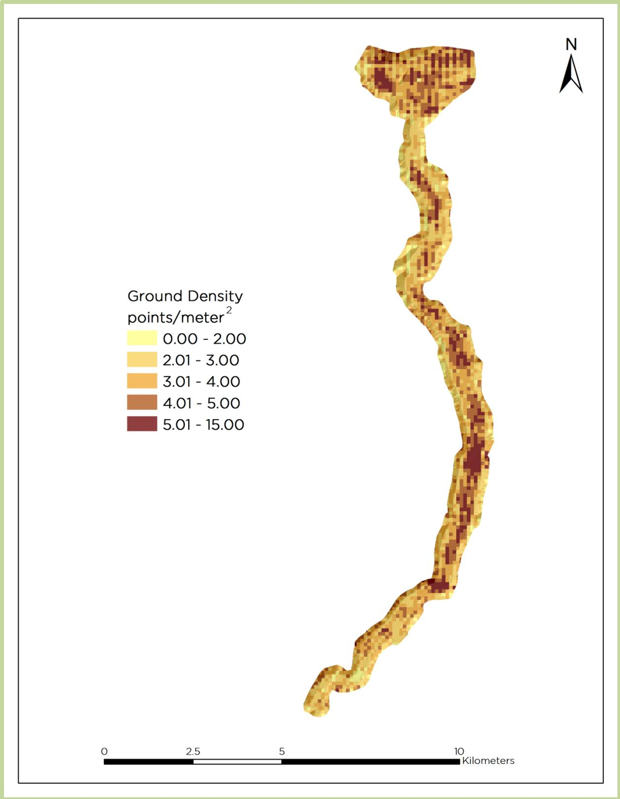
Figure 7: Ground density map for the Rock Creek LiDAR site
