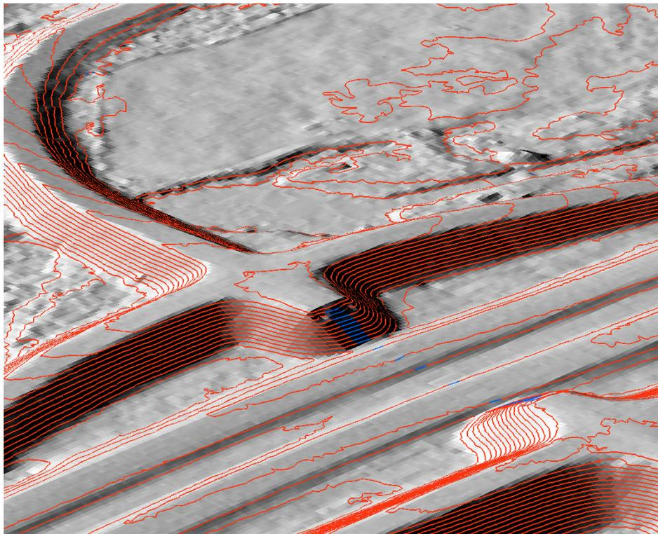
**Figure 3: Contours draped over the Rock Creek LiDAR bare earth elevation model. Red contours represent high confidence while the blue contours represent lower confidence.**
