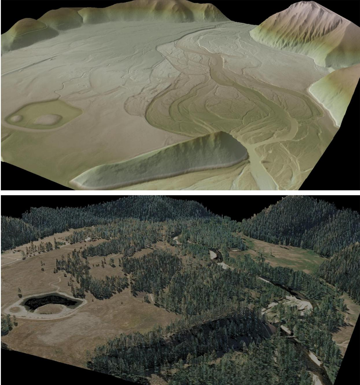
**Figure 10: The top image is the LiDAR bare earth model colored by elevation looking south up Rock Creek. The bottom image is the 3D LiDAR point cloud colored with NAIP imagery.**
