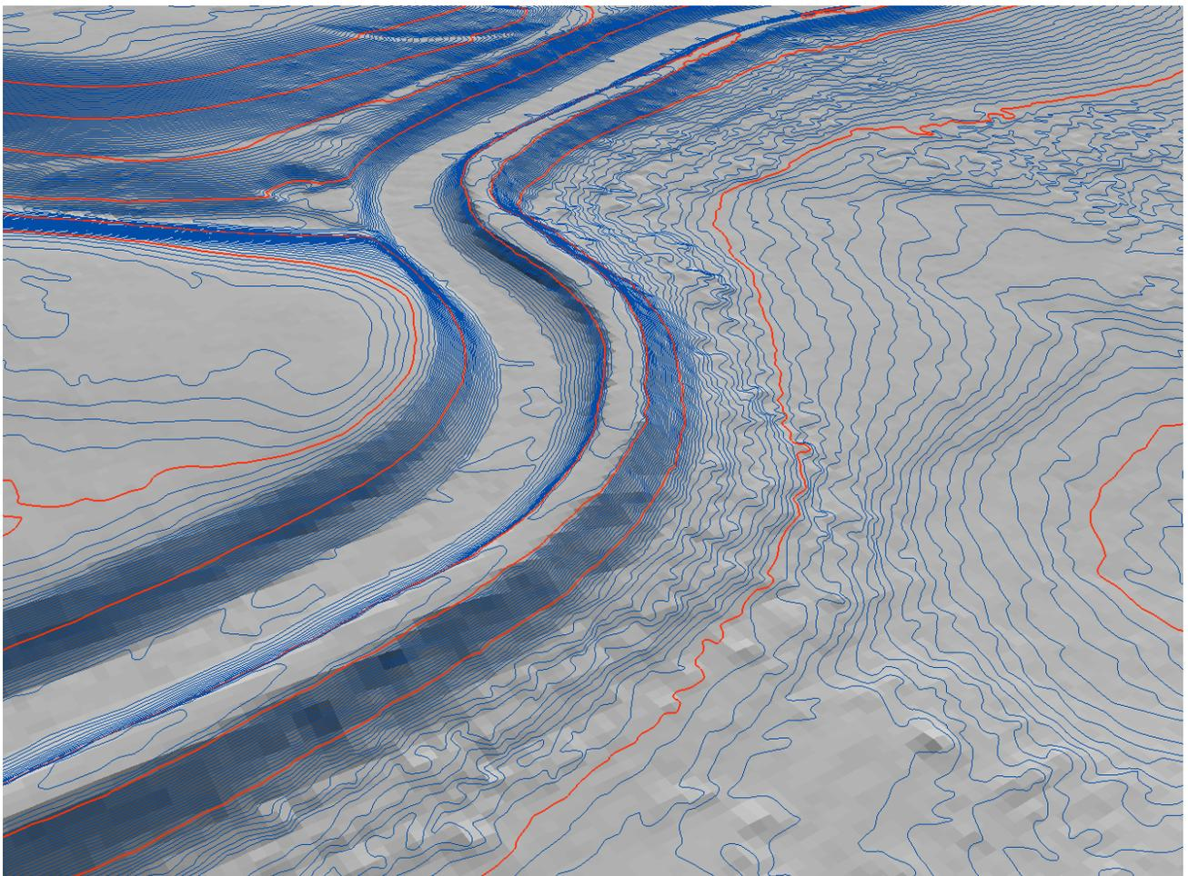
**Figure 4: Contours draped over the Saint Mary Canal bare earth elevation model. Blue contours represent basic 0.5 foot intervals while the red contours represent major 10 foot intervals.**
