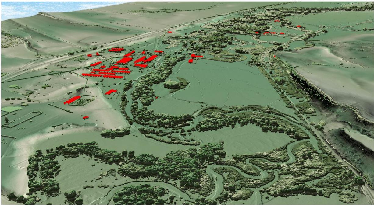
**Figure 5: This image shows a view of the building classification in the Musselshell and Wheatland Counties site, created from the bare earth model colored by elevation, and overlaid with the above-ground point cloud colored by point classification.**
