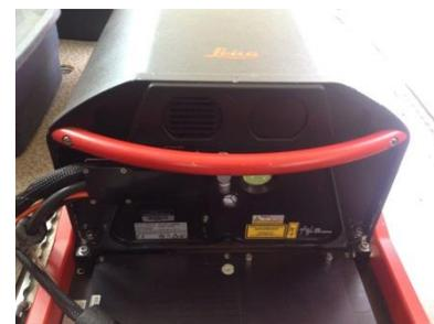
**Leica ALS80 LiDAR sensor**
