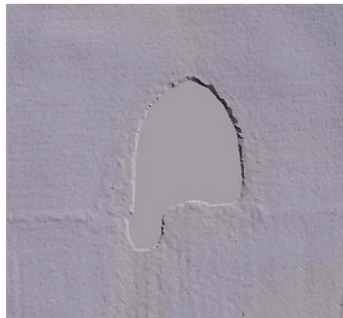
Figure 4.2 reflects a DEM generated from original LiDAR bare earth point data prior to the hydrologic flattening process. Note the "tinning" across the lake surface.
