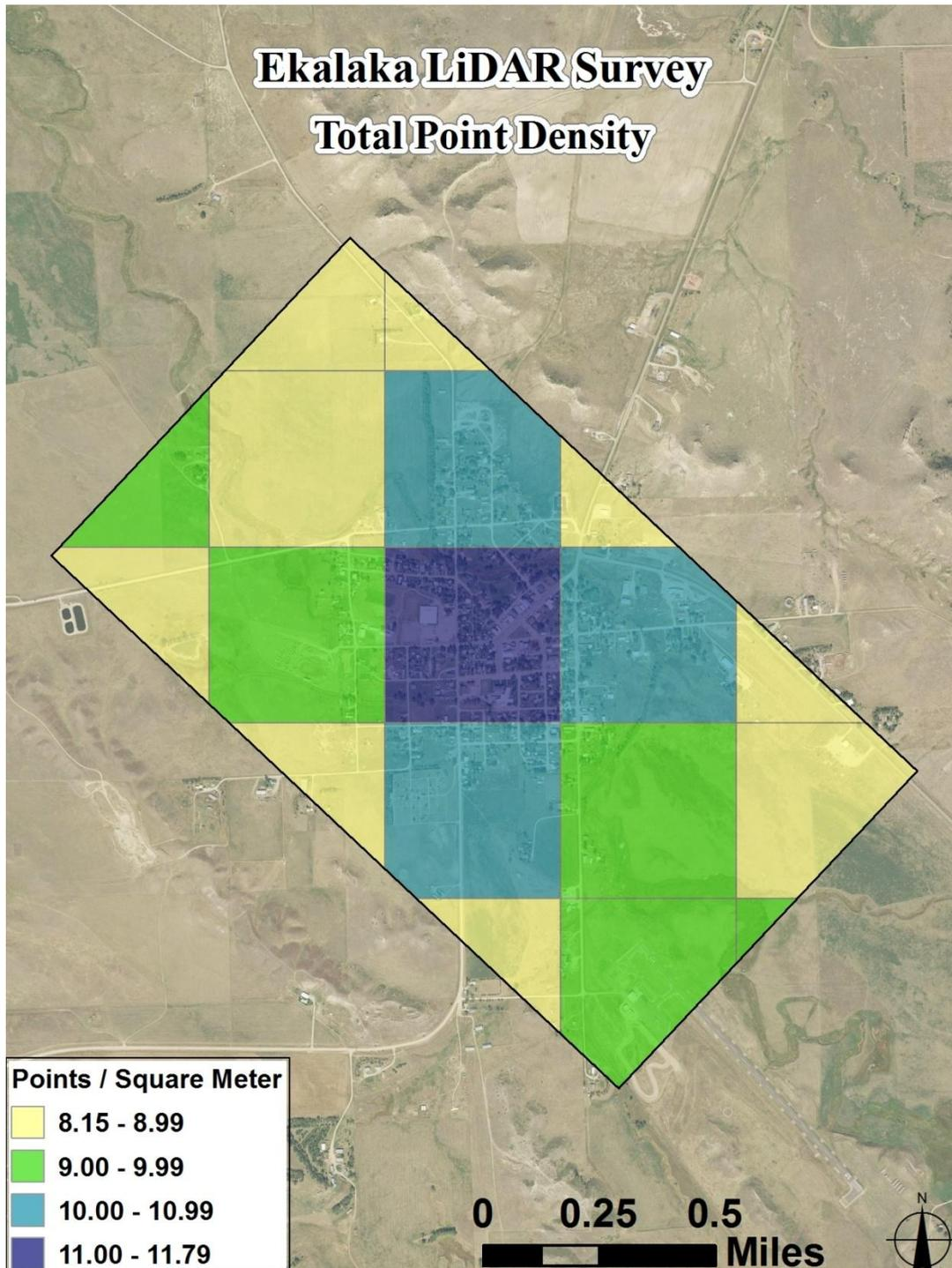
The following two exhibits show the density of **ground classified points**. Factors such as vegetation, water, and buildings will reduce the density of points classified to the ground. For the Ekalaka project, an average of **6** ground classified points per square meter was achieved.
