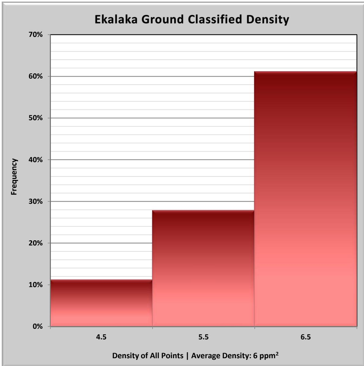
**Exhibit 15:** Ground Classified Laser Point Density by Tile, points/m<sup>2</sup>
