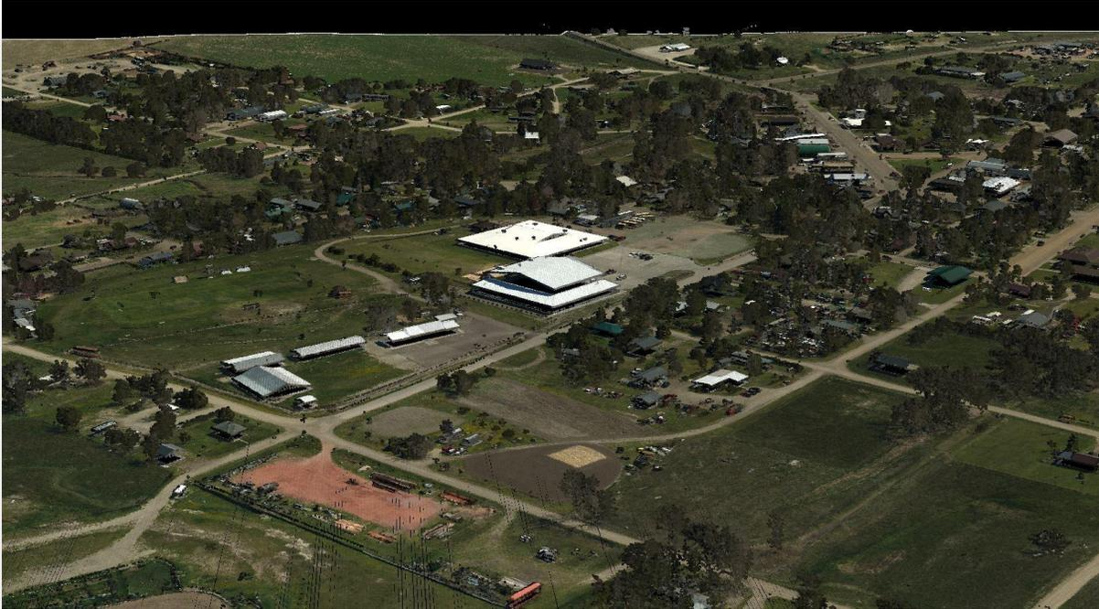
**Exhibit 17:** LiDAR point cloud colored by elevation and intensity values
