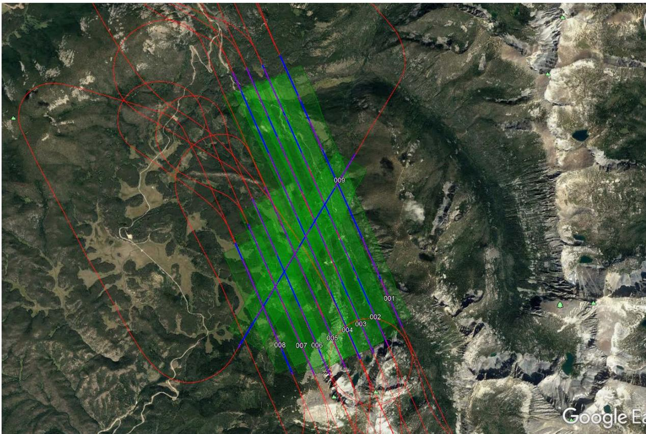
Figure 2. A total of nine flight lines were executed for LiDAR acquisition. Eight parallel lines and a ninth passing through the others.
