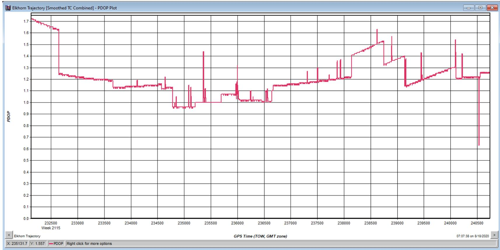
Figure 5. PDOP observed during data collection flight.
