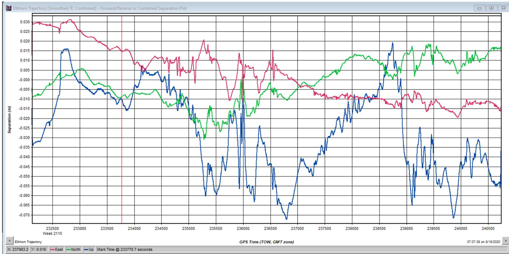
Figure 6. Linear separation between GNSS and INS trajectories. Red, green, and blue show easting, northing, and elevation separations, respectively.
