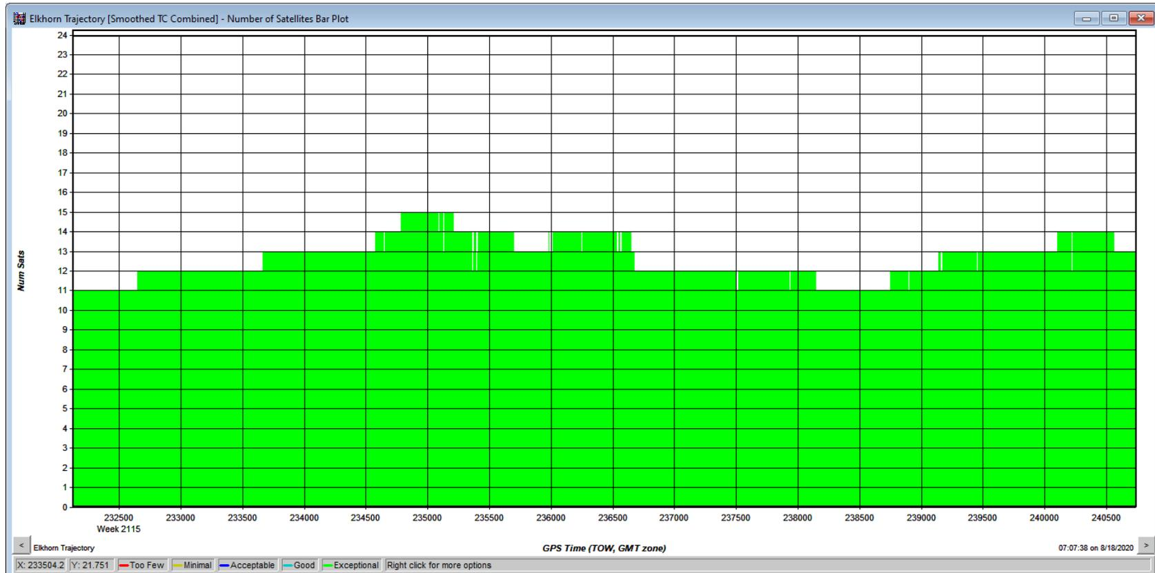
Figure 4. GNSS satellite quantities observed during data collection flight.
