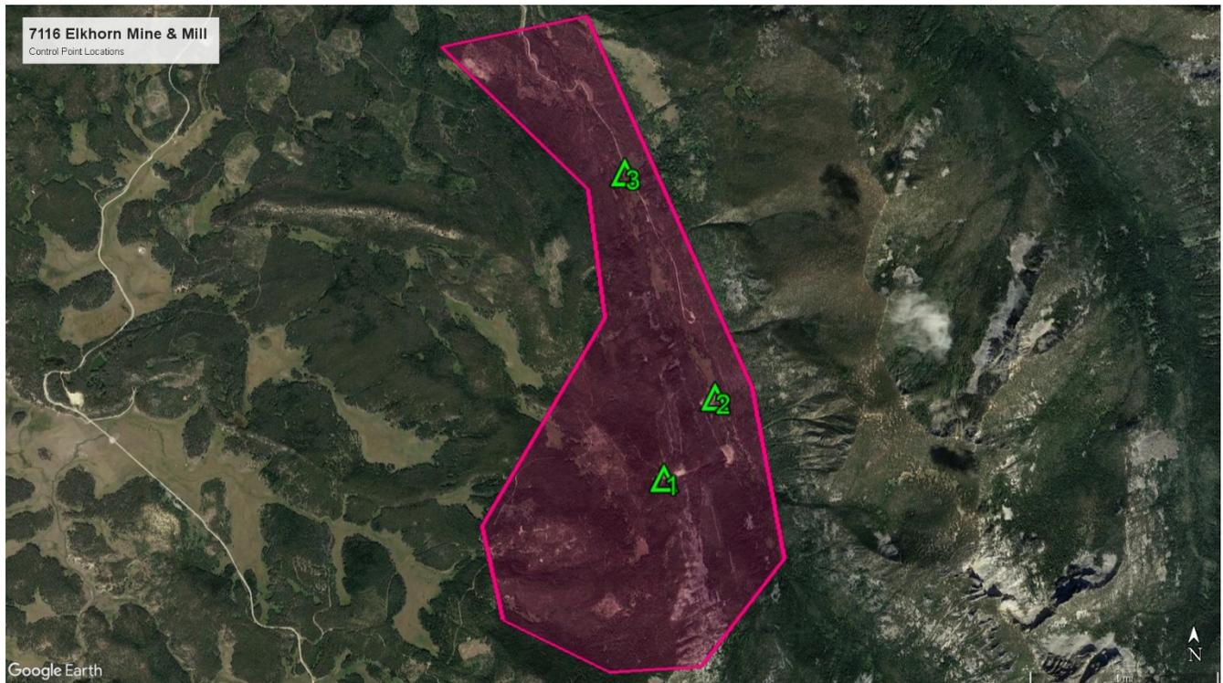
Figure 3. Control points set for LiDAR acquisition. Control points 1 and 3 were used to control LiDAR products. Control point 2 was set for future survey related tasks.
