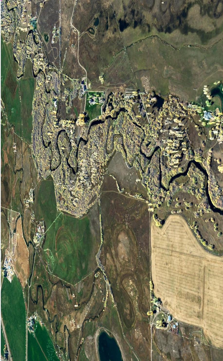
Figure 11: View looking northeast across a meandering river in the central part of the Dillon AOI. The image was created from the LIDAR bare earth model overlaid with the above-ground point cloud and USDA NAIP imagery.
