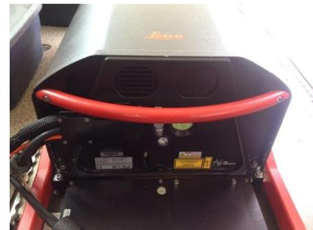
**Leica ALS80 LiDAR sensor**
