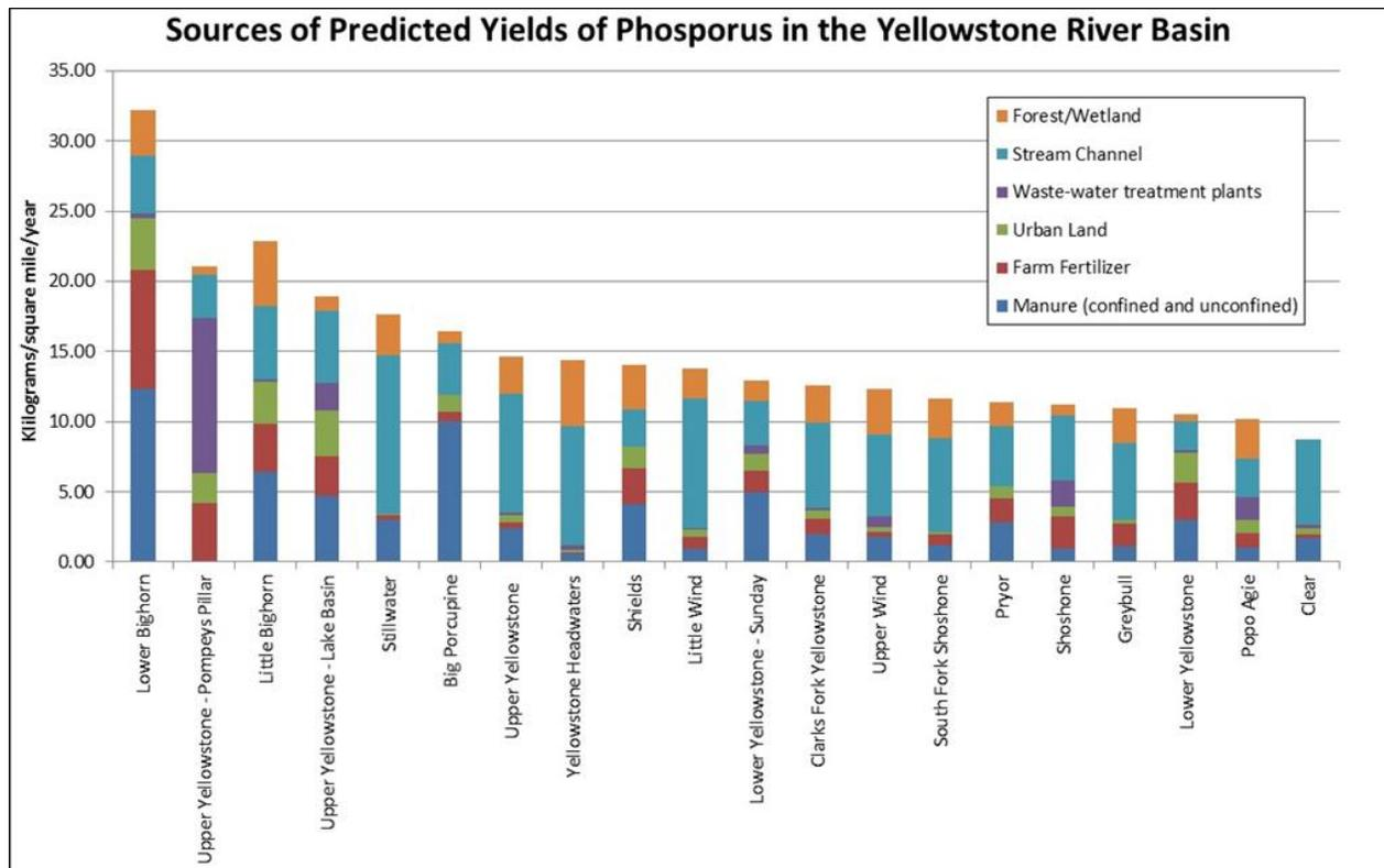
**Figure 4-97 Sources of the predicted yields of delivered aggregated phosphorus yields by hydrologic units within the Yellowstone River Basin**
