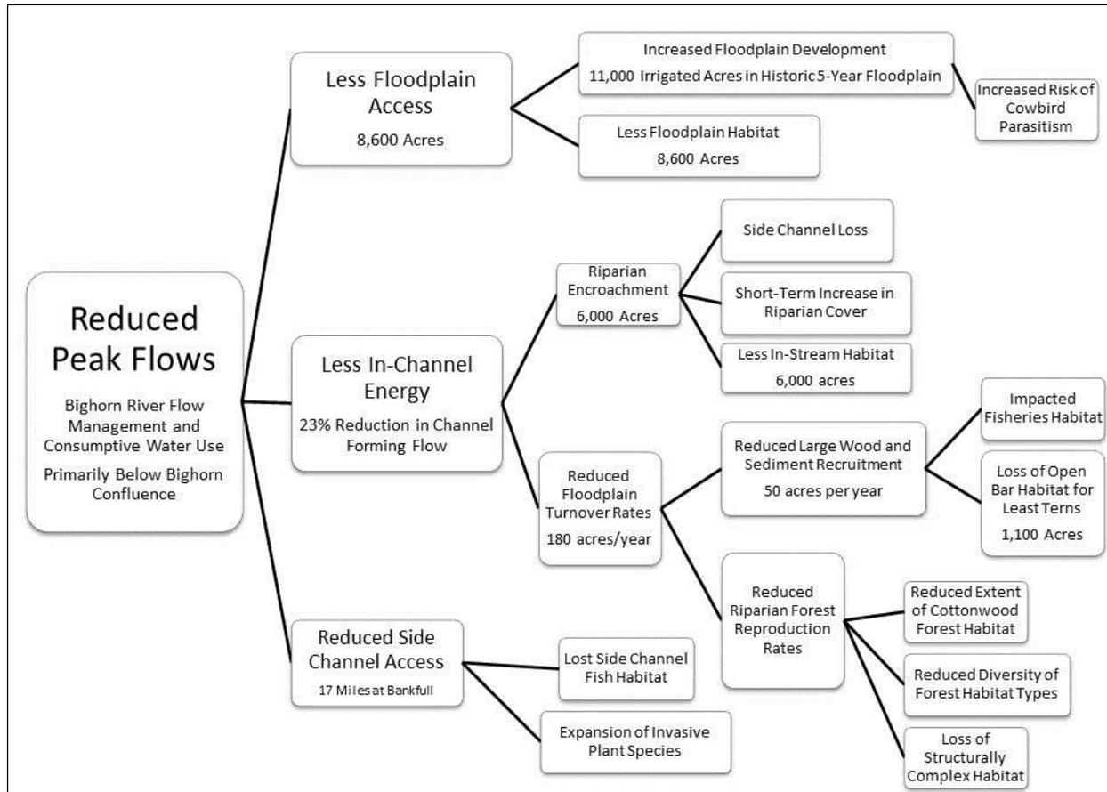
**Figure 7-2 Schematic diagram showing cumulative effects from reduced peak flows**
