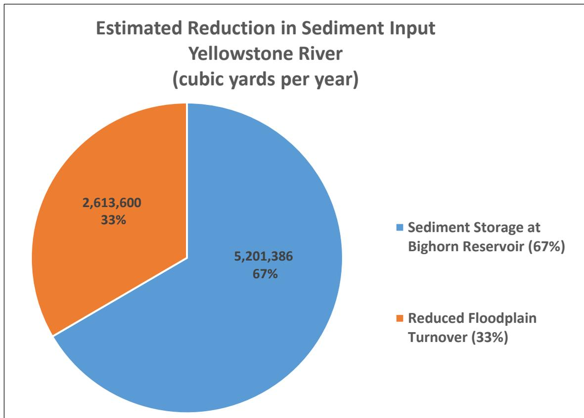
**Figure 4-89** Estimated reduction in sediment delivery from Bighorn Reservoir Storage and Mainstem Yellowstone Bank Erosion (reservoir storage volumes from USBOR 2010b)
