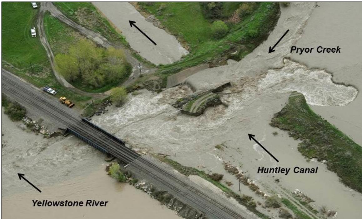
**Figure 4-22** View of active flanking of Huntley Canal tunnel by Pryor Creek during 2011 flood
