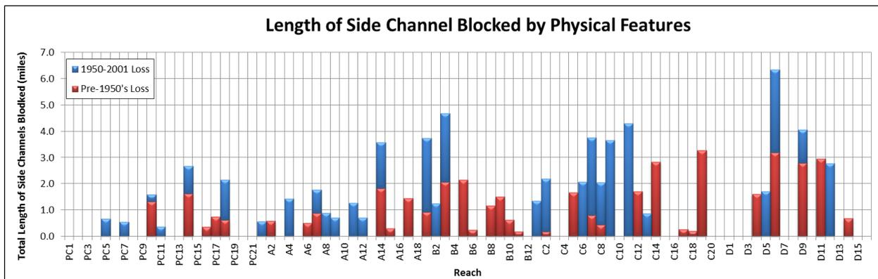
Figure 4-67 Total side channel loss due to blockages, pre- and post-1950s
