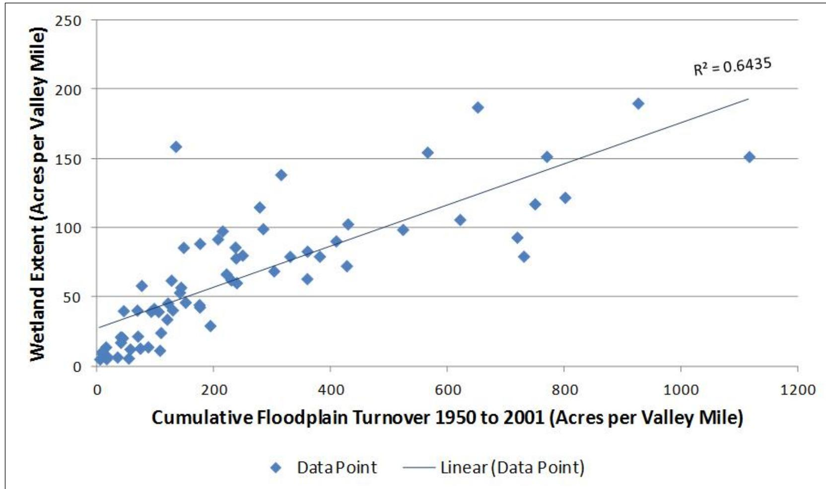
**Figure 4-138 Relationship of wetland density to the cumulative floodplain turnover (loss and gains) for all channel types**
