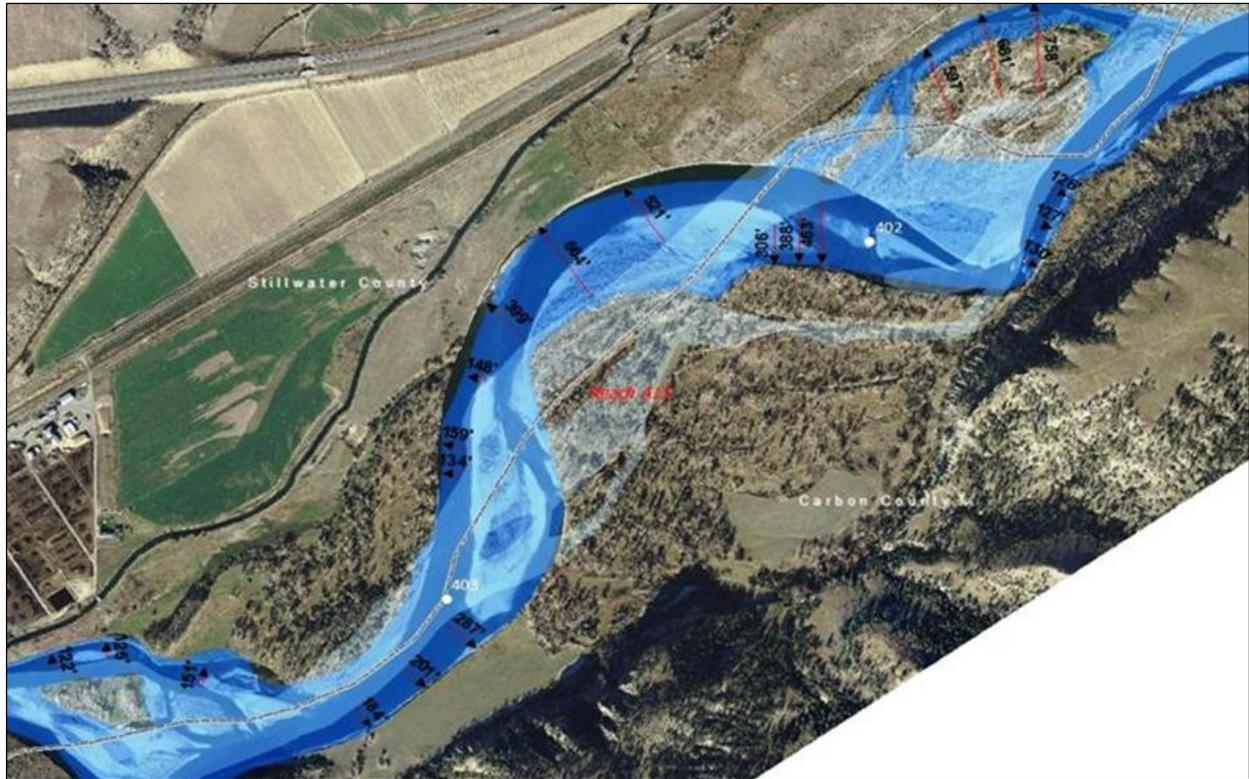
**Figure 4-120 Comparison of 1950 to 2011 channel location in Reach A15**
