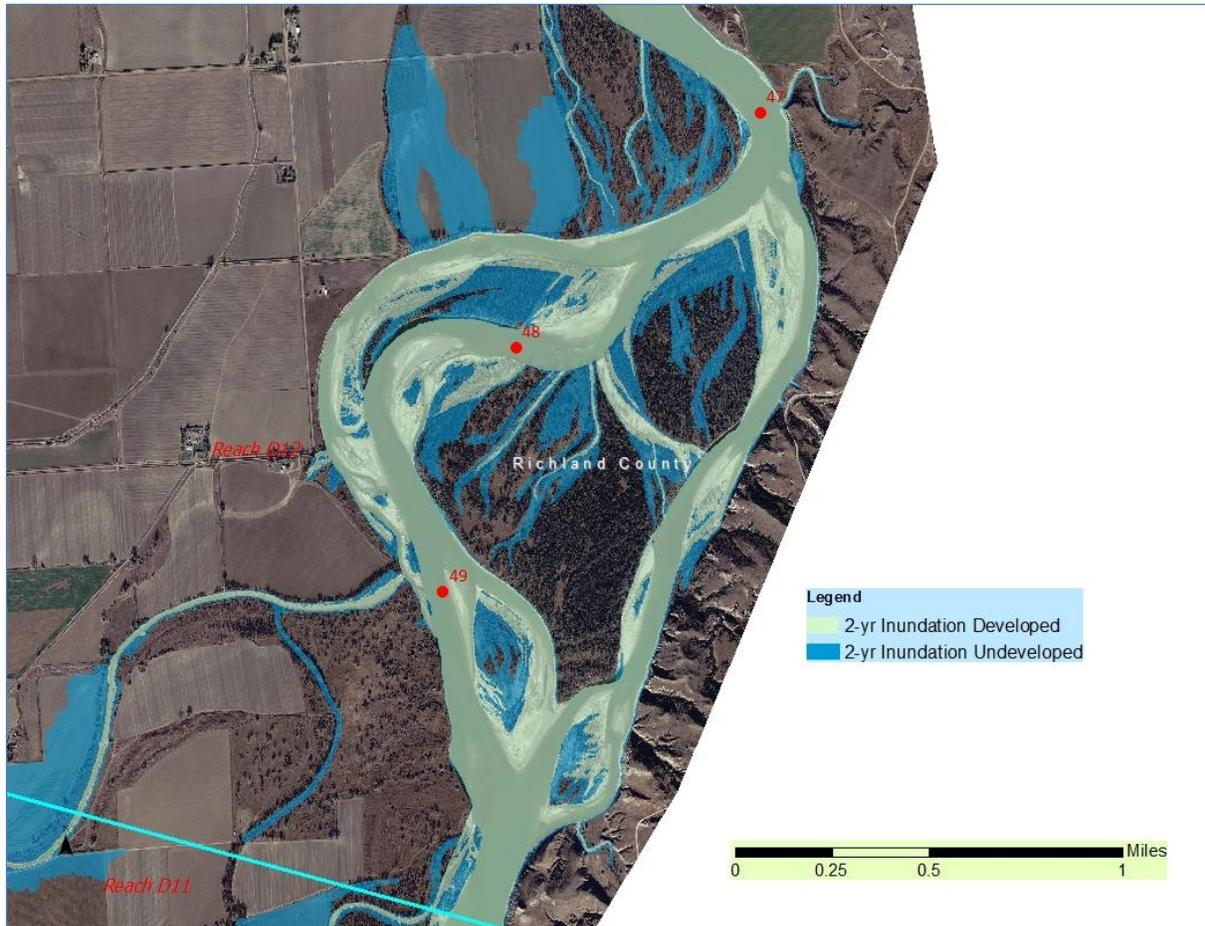
**Figure 4-62 Hydraulic modeling results showing inundated area for 2-year undeveloped and 2-year developed conditions, Reach D12**
