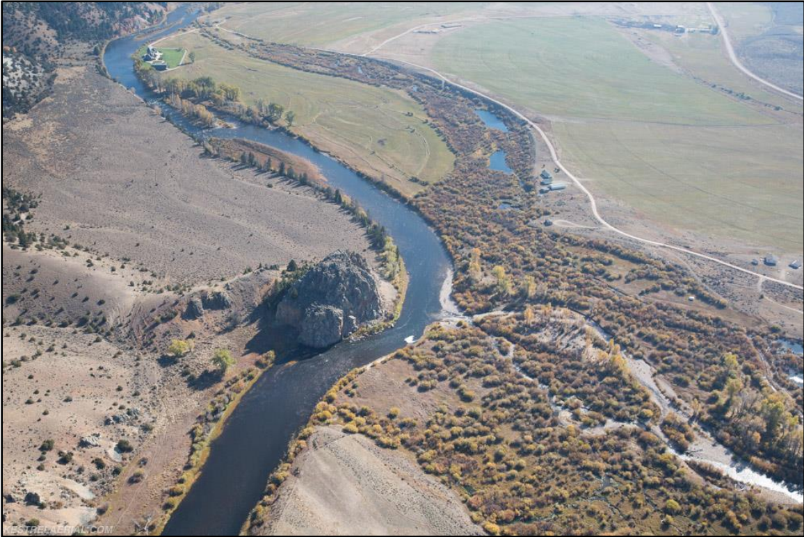
Figure 47. View downstream of Reach BH9 past mouth of Wise River showing avulsion path that extends behind residence. (Kestrel)
