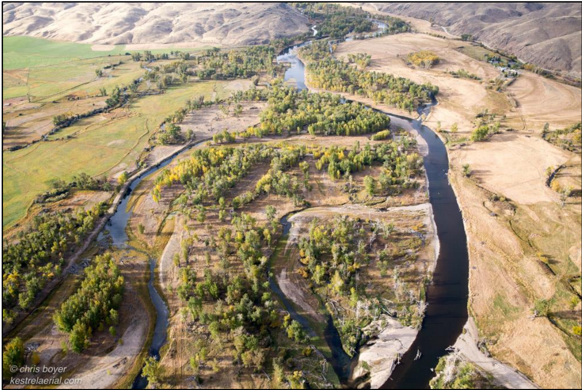
Figure 66. View upstream of avulsion site in Reach BH1; the decaying 1979 channel is to left.
