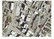
Digital orthoimagery are georeferenced images of the Earth's surface. Displacement of objects has been removed for sensor distortions and orientation and for terrain relief. Many geographic features, including those that are part of the Framework, can be interpreted and compiled from an orthoimage. Orthoimages can also serve as a backdrop to reference the results of an application to the landscape.
