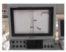
directly to the computer system. It was calibrated using several measurements from an Odom "Digibar" velocimeter.
