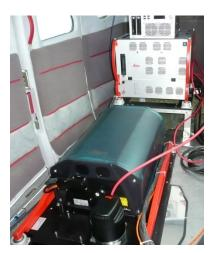
Leica ALS70 LiDAR sensor
