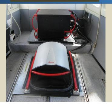
ALS60 LiDAR sensor installation
