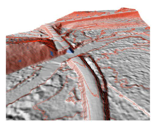
Figure 3: Contours draped over the Missoula County LiDAR bare earth elevation model. Red contours represent high confidence while the blue contours represent lower confidence.
