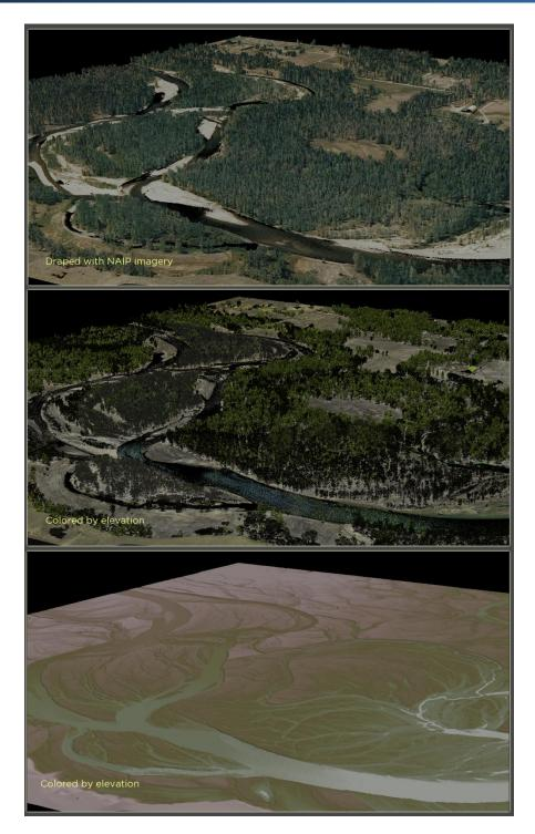
Figure 10: View looking east at the Bitterroot River. The top image is the 3D LiDAR point cloud draped with NAIP imagery, the center image is the LiDAR point cloud colored by elevation, the bottom image is the gridded bare earth model colored by elevation.
