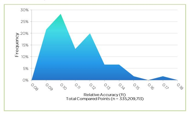
Figure 9: Frequency plot for relative accuracy between flight lines
