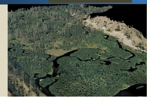
View looking north at Owl Creek. The 3D LiDAR point cloud is draped with NAIP imagery.
