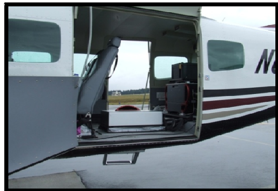
The Cessna Caravan is a stable platform, ideal for flying slow and low for high density projects. The Leica ALS50 sensor head installed in the Caravan is shown on the left.
