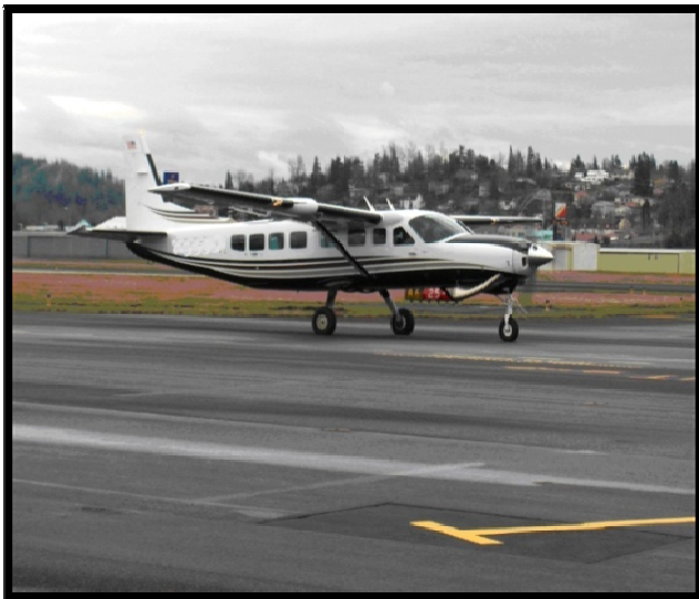
The Cessna Caravan is a stable platform, ideal for flying slow and low for high density projects. The Leica ALS50 sensor head installed in the Caravan is shown on the left.
