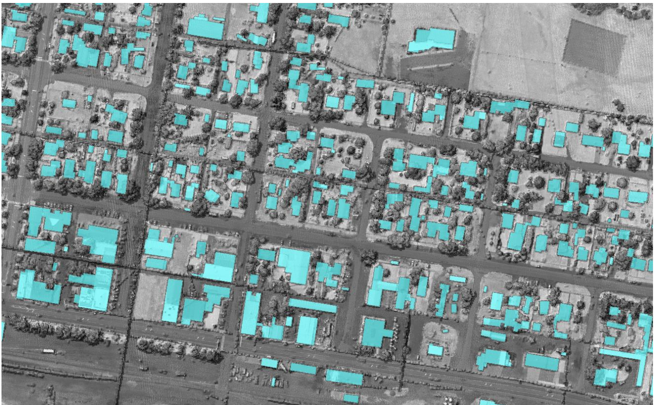
Figure 3: This aerial view of the lidar point cloud is colored by intensity and is overlaid with the 3D building footprint in the Deer Lodge County project area.
